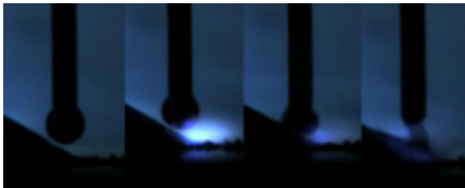
Fig. 14. Experimental run showing single peak short occurring during base time of the one pulse cycle at peak current 280 A, base current 60 A, peak time 2 ms, and base time 27 ms
