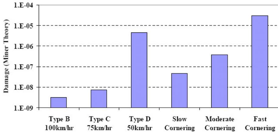
Fig. 14. Column chart of fatigue damage per kilometer of straight (three types), cornering and braking maneuvers
