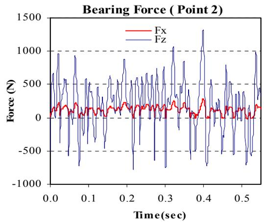
Fig. 6. Time history of loads in straight driving on road type C
