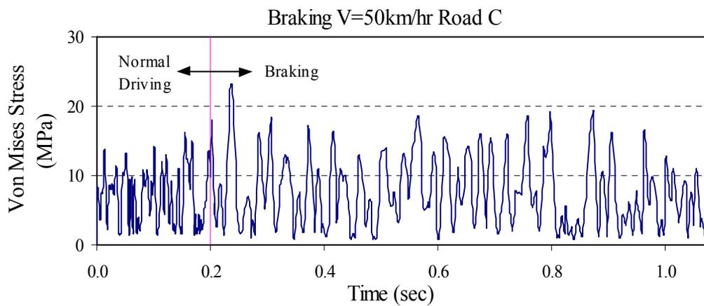
Fig. 13. Time history of Von-Mises stress in braking maneuver
