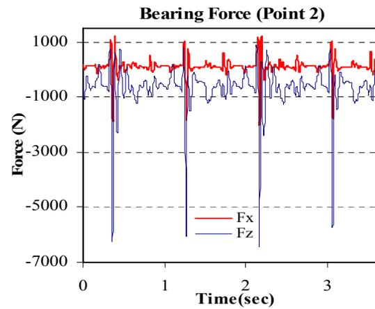
Fig.7. Time history of loads in driving on simple pothole
