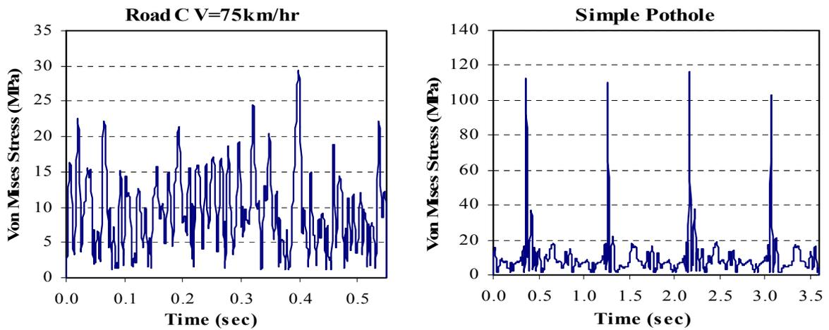
Fig. 11. Time history of Von-Mises stress in straight driving on road type C and simple pothole
