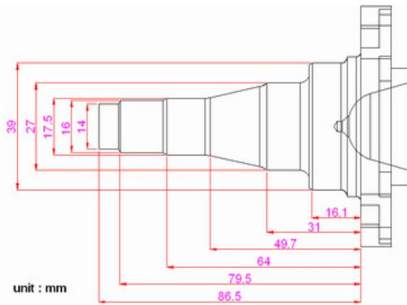
Fig. 4. Details and dimensions of spindle
