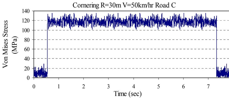
Fig. 12. Time history of Von-Mises stress in fast cornering cycle (straight- cornering- straight)
