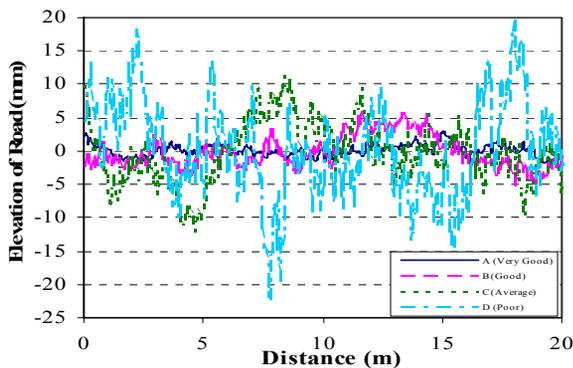
Fig. 1. Sample road profile of ISO standard roads [5]
