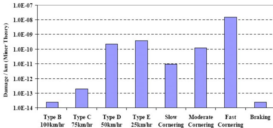
Fig. 15. Column chart of fatigue damage share of different maneuvers in 200000km driving
