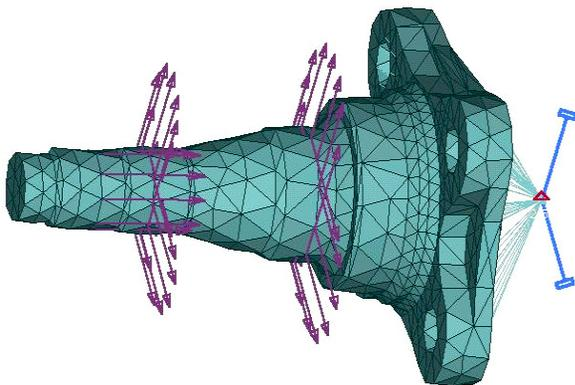
Fig. 10. Spindle and its FEM model
