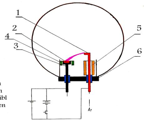
Fig. 1b. schematic diagram of Ion coating element.
