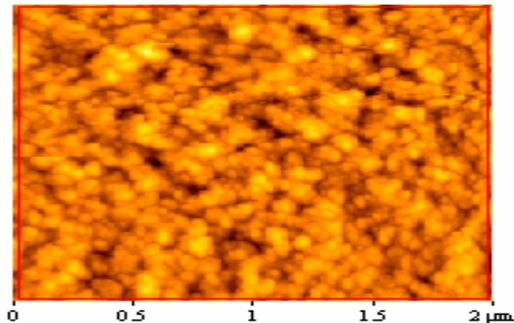
Fig 7. Two-dimensional AFM image of  $TiC_{0.47}N_{0.53}$  coating on glass.
