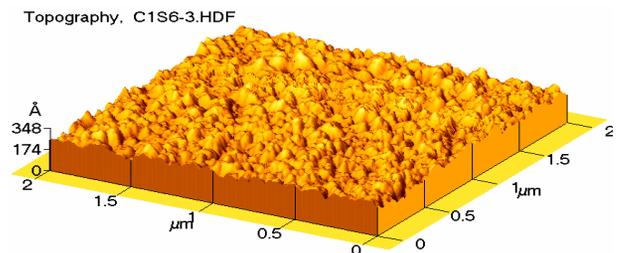
Fig. 6. three dimensional AFM image of  $TiC_{0.47}N_{0.53}$  coating on glass.
