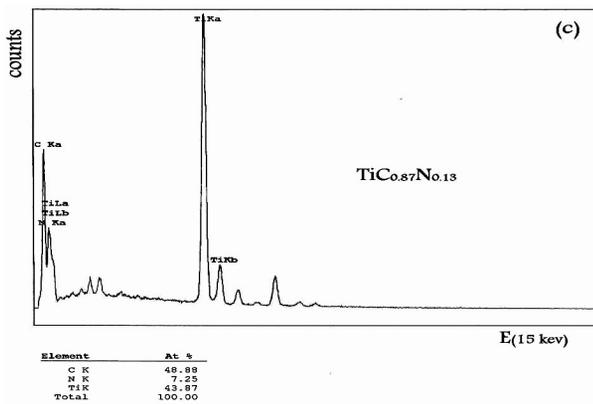
Fig 5. EDX analysis of  $TiC_xN_y$  coatings on steel 316.
