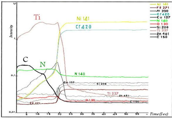
Fig. 3b. GD-OES analysis of TiC<sub>0.58</sub>N<sub>0.42</sub> on stainless steel 316.
