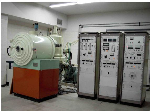
Fig. 1a. A view of Ion coating apparatus
