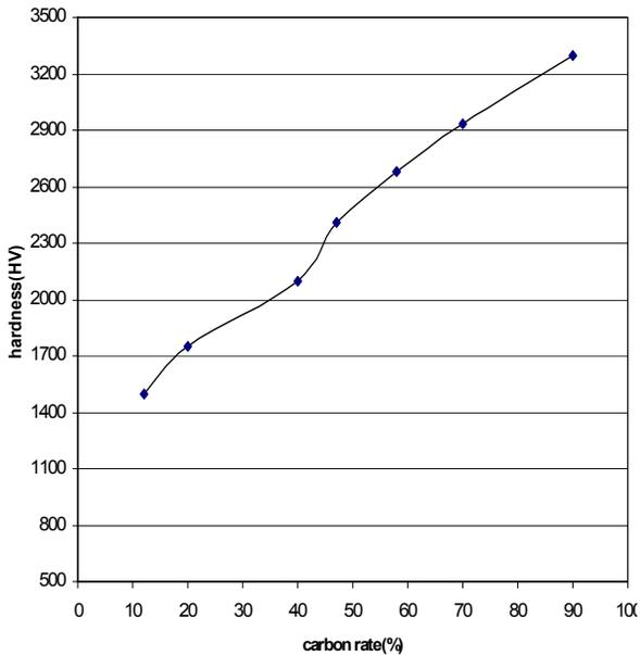
Fig. 9. micro hardness of Ti(C, N) with different carbon content.
