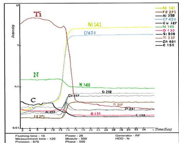
Fig. 3a. GD-OES analysis of TiC<sub>0.20</sub>N<sub>0.80</sub> on stainless steel 316.
