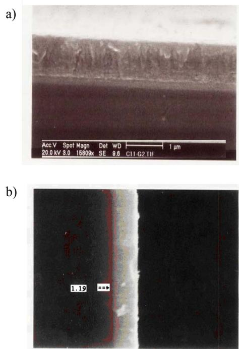
Fig 8. SEM micrographs of  $TiC_{0.47}N_{0.53}$  deposited on glass substrate with  $1.19\mu$  thickness.
