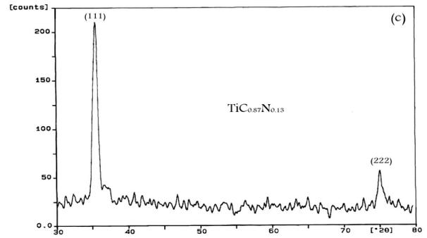
Fig. 4. X-Ray diffraction patterns of TiC<sub>x</sub>N<sub>y</sub> coatings on glass.
