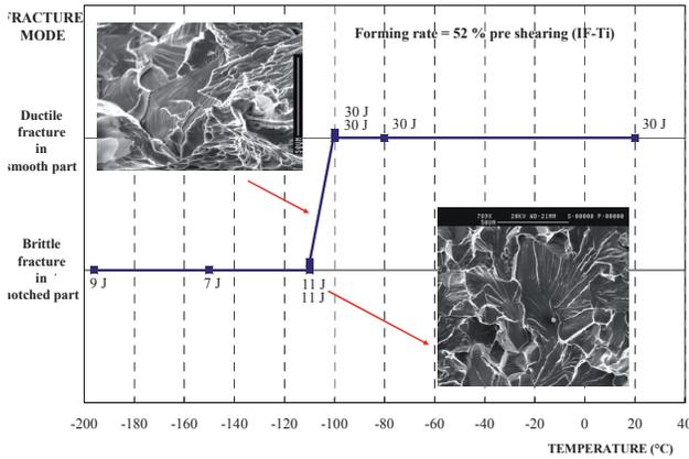
Fig. 2c. Ductile-brittle transition (DBTT) curves of fracture mode obtained by simulated crash test at the conditions of the forming rate of  $\epsilon = 52\%$
