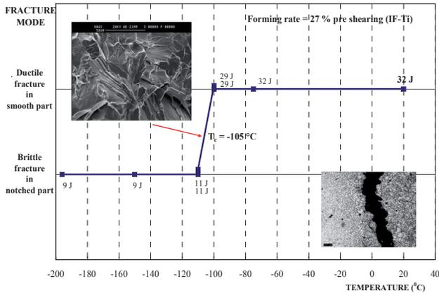
Fig. 2b. Ductile-brittle transition (DBTT) curves of fracture mode obtained by simulated crash test at the conditions of the forming rate of  $\epsilon = 27\%$
