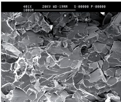
Fig. 3a. SEM microphotographs of the non-preformed a specimens under the chock (base metal),  $\epsilon = 0\%$  (test= -150°C)
