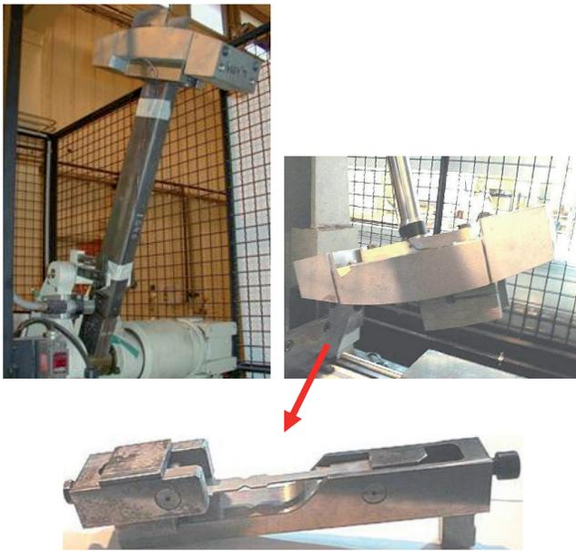
Fig. 1c. Simulated crash test installation of the assembly with hammer and support adapted to the double cutter and specimen for the testing of the steels (capacity of the assembly: 650J)
