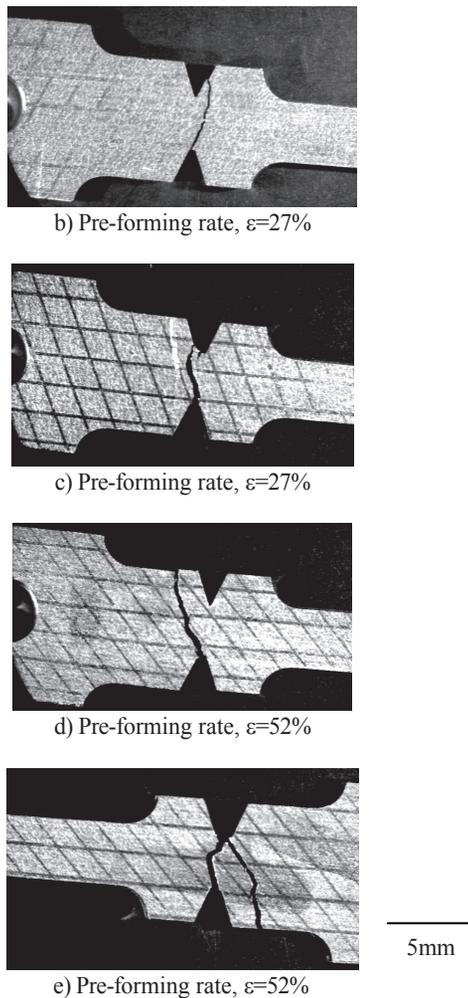
Fig. 4b-e. Fracture macrophotographs of the specimens under chock at 27 and 52 % of pre-forming conditions
