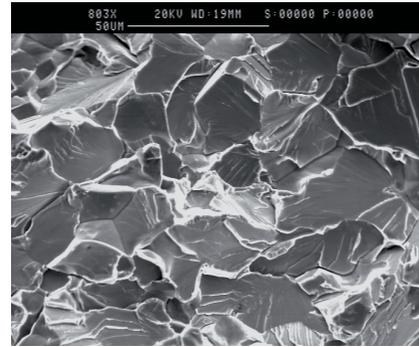
Fig. 3b. SEM microphotographs of the pre-formed specimens under the chock (base metal),  $\epsilon=27\%$  (test= -150°C)
