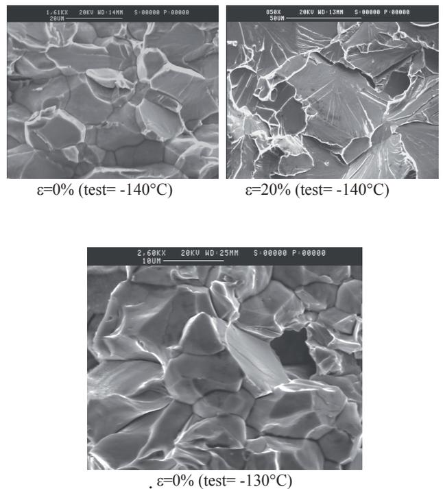
Fig. 6. SEM microphotographs of the non-preformed and pre-formed tailored blanks under the chock, IF-Ti
