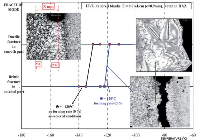
Fig. 5. Ductile-brittle transition (DBTT) curves of fracture mode obtained by simulated crash test of the tailored blanks
