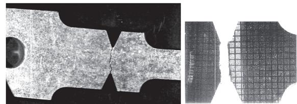
Fig. 4a. Fracture macrophotographs of the specimens under chock at 0% of pre-forming rate conditions
