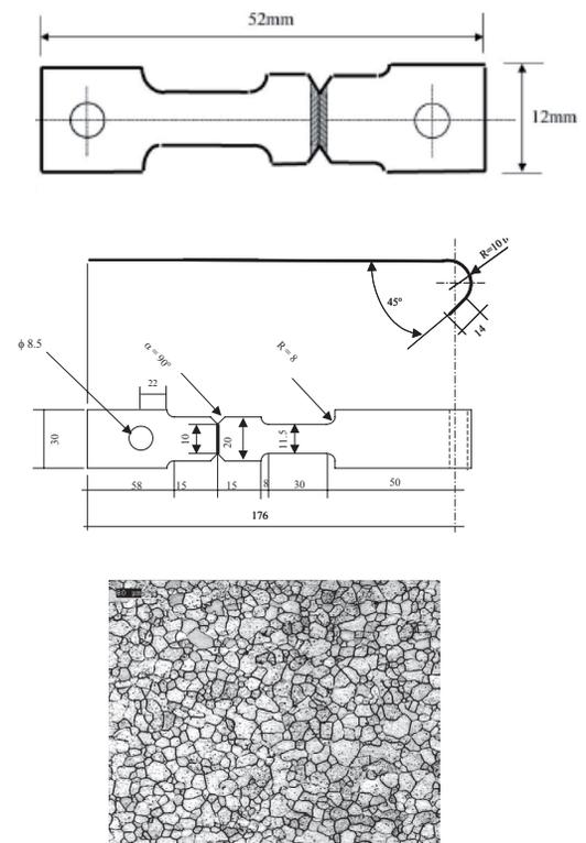
Fig. 1b. Sample geometries and microstructure of IFS used in simulated crash test applications
