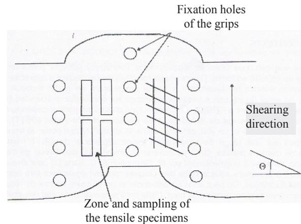
Fig. 1a. Schematic of specimen device containing a homogenous sheared zone allowing the sampling for crash test
