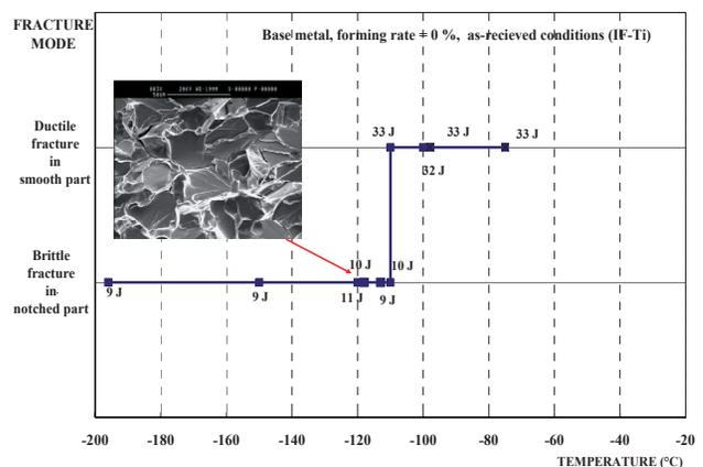
Fig. 2a. Ductile-brittle transition (DBTT) curves of fracture mode obtained by simulated crash test at the conditions of the forming rate of  $\epsilon = 0 \%$
