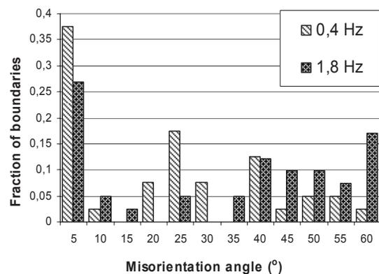
Fig. 8. Misorientation angles distributions developed in Cu after deformation at 0.4 Hz and 1.8 Hz
