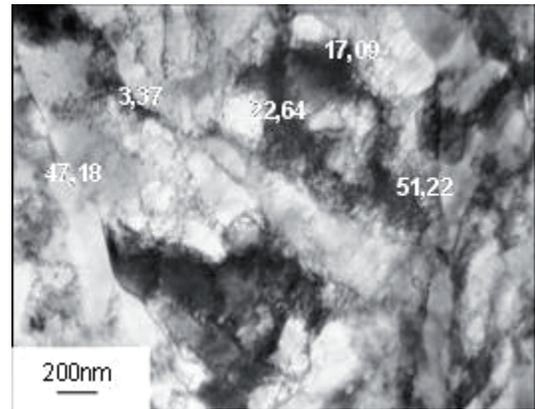
Fig. 2. Development of cells/subgrains structure in Cu deformed at 0.4 Hz. Dislocation cell structure with small and higher value of misorientation. On the left side the grain boundary indicating mobility
