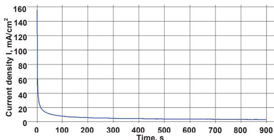
Fig. 3. Change of anodic current in a function of time for electro-polished and chemically passivated with carbon layer samples
