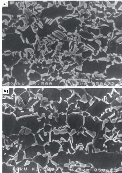
Fig. 5. SEM microstructures of samples after annealing at 850°C/60s and isothermal holding at: a) 500°C/600s – sample 1; b) 400°C/600s – sample 3
