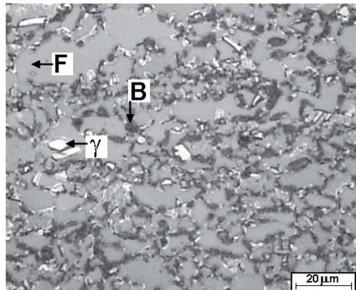
Fig. 6. Color etching of TRIP type microstructure of the sample 1 isothermally annealed at 500°C/600s
