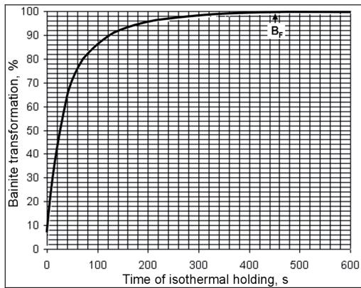
Fig. 3. Kinetics of bainite transformation during isothermal holding 450°C/600s of the sample no 2
