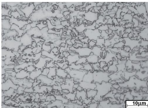
Fig. 4. TRIP type microstructure of the sample 2 austenitized at 850°C/60s, isothermally annealed at the temperature 450°C/600s
