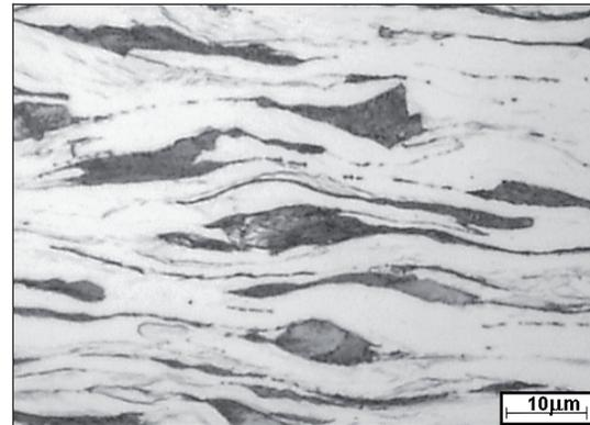
Fig. 1. Band ferrite-pearlite microstructure of the cold-rolled sample in the initial conditions, magn.1000x
