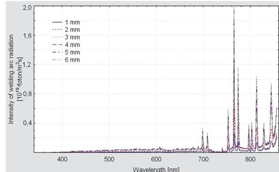
Fig. 1. Effect of the arc length on the arc light spectrum. The welding current 200 A, the arc length in the range of 1÷6 mm, the shielding gas – 100 %Ar, wavelength in the range of 340÷860 nm
