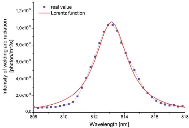
Fig. 2. Calculated line profile of the wavelength 813,22 nm compared with measured values. The Lorentz function with the characteristic qualities
