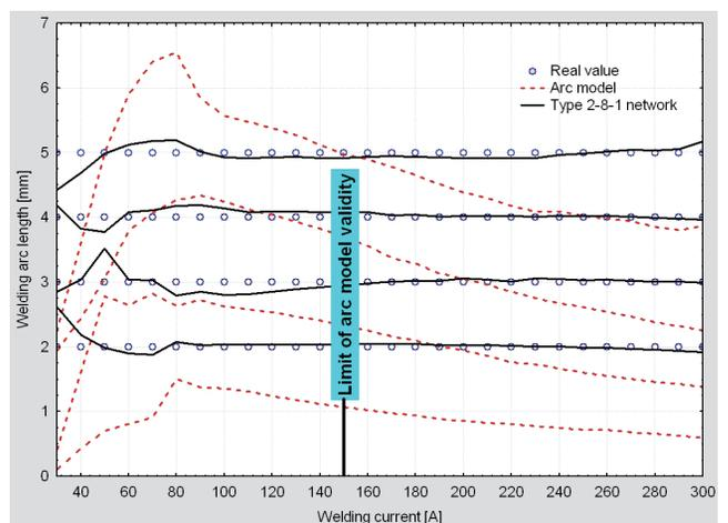
Fig. 4. Scatter diagram for calculation results obtained by using the welding arc model, artificial neural network in comparison with the real values of the welding arc length
