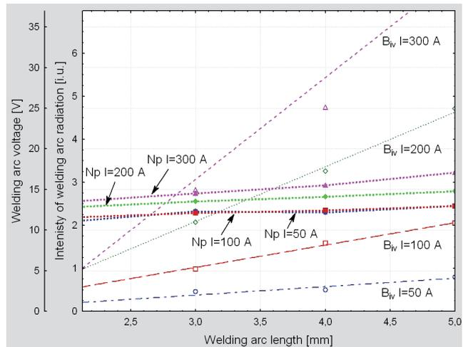
Fig. 3. The influence of the welding arc length on the radiation intensity ( $B_{iv}$ ) and the arc voltage ( $N_p$ ) at the welding current in the range of 50÷300 A. The Argon as shielding gas
