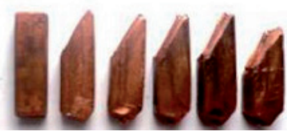
Fig. 2. Copper samples after individual passes with using the ECAP technology
