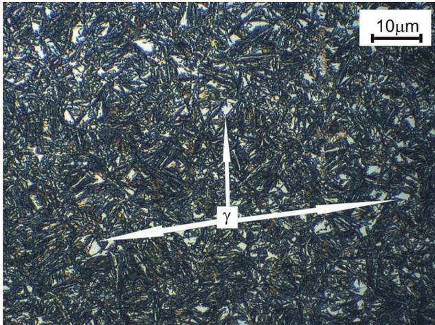
Fig. 2. Structure of the ferritic bainite with the retained austenite for the steel isothermally quenched to a temperature of 250°C
