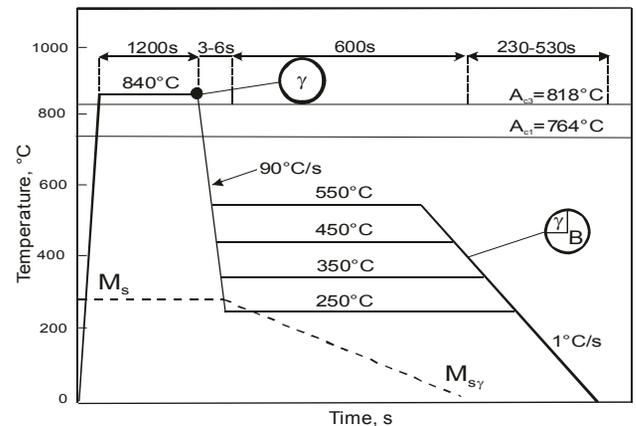
Fig. 1. Heat treatment of the investigated steel;  $M_s$  – martensite start temperature of the steel,  $M_{s\gamma}$  – martensite start temperature of the austenite with increased carbon concentration
