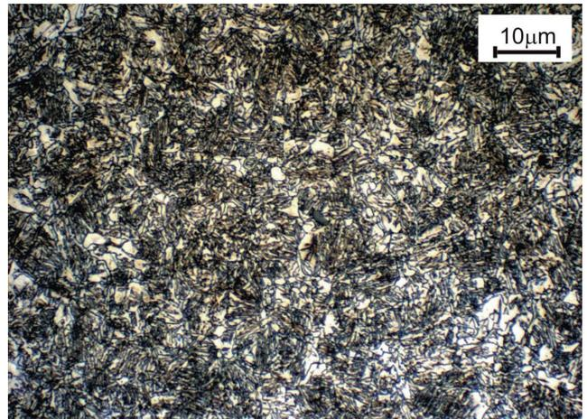
Fig. 3. Structure of the upper bainite with the retained austenite for the steel isothermally quenched to a temperature of 450°C
