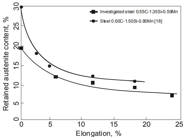
Fig. 5. A change in the retained austenite fraction as a function of the elongation of the specimen
