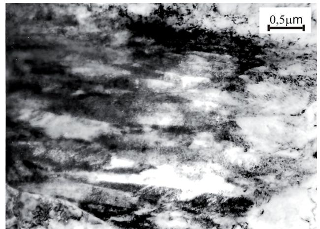
Fig. 4. Retained austenite as films between laths of the ferritic bainite
