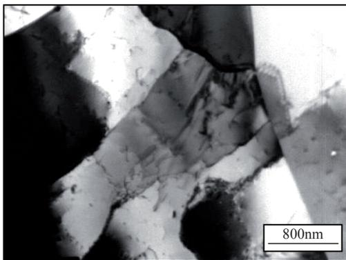
Fig. 4. Substructure of the alloy after compression at 900°C
