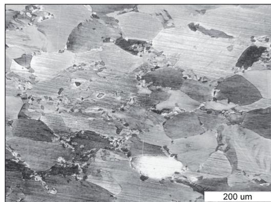
Fig. 6. Structure of the FeAl alloy after cold compression and annealing at 700°C
