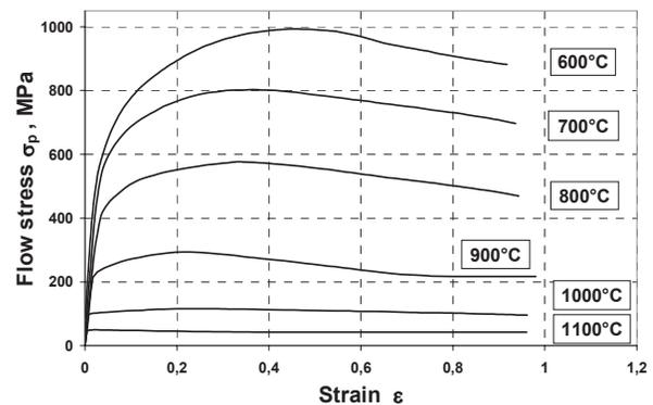
Fig. 2. Stress strain curves for Fe-38Al alloy deformed at temperature 600 - 1100°C with a rate  $0.1\text{s}^{-1}$
