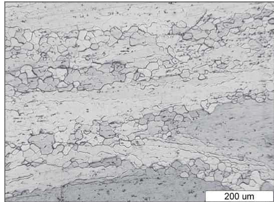
Fig. 5. Structure of the alloy after compression at 1000°C
