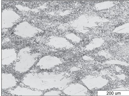
Fig. 3. Structure of the alloy after compression at 900°C
