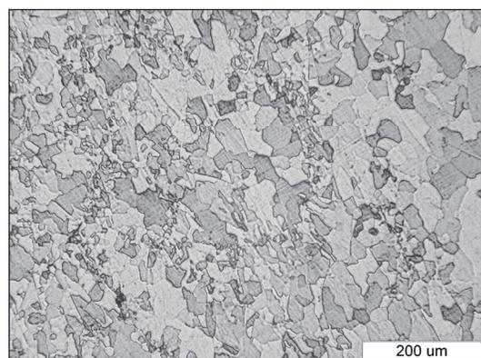
Fig. 7. Structure of the FeAl alloy after cold compression and annealing at 800°C
