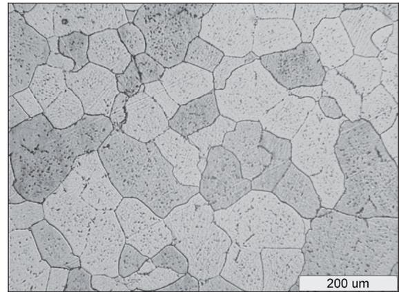
Fig. 1. Microstructure of the Fe-38Al alloy after homogenization annealing at 1000°C for 48h, followed by cooling with furnace
