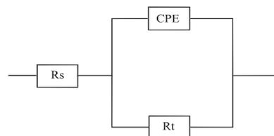
Fig. 5 An equivalent circuit model of heat treatment  $\text{Co}_{77}\text{Si}_{11.5}\text{B}_{11.5}$  samples in temperature range 723K to 923K at corrosion potential in 3% NaCl solution, where  $R_s$  – solution resistance,  $R_t$  - charge transfer resistance, CPE – capacitance of constat phase element
