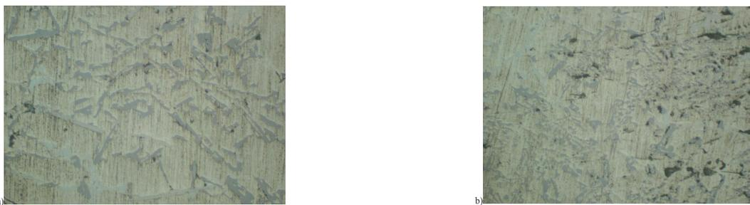
Fig. 4. AlSi11 micrographs taken along the radius of horizontal section of the sample casting. As can be seen dispersion of the eutectic components grows from the center to the surface of the casting. a), casting center, b) casting surface; a) Microstructure from center region, b) Microstructure near the mould region
