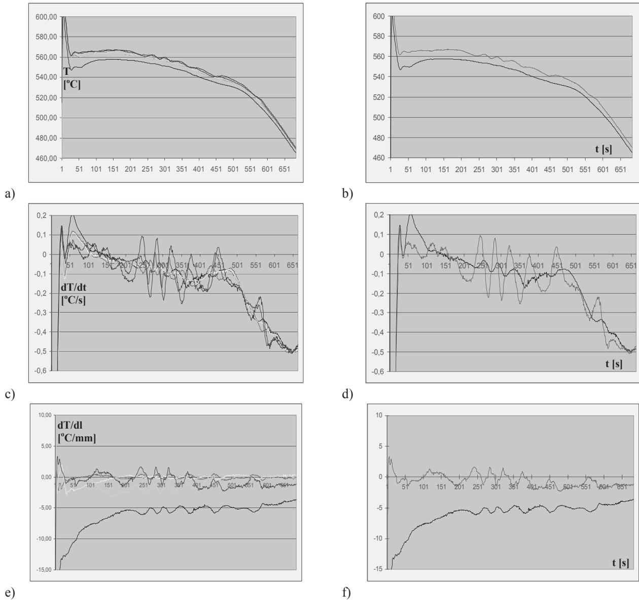
Fig. 3. Relations:  $T=f(t)$ ,  $dT/dt=f(t)$  and  $dT/dl=f(t)$  obtained for six thermocouples placed along the radius of sample casting (fig. a, c, e) and for extreme positions, that is in the center and near the surface of the mould (fig. b, d, f)
