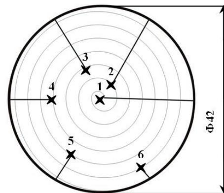
Fig. 2. Distribution of the thermocouples on casting section
