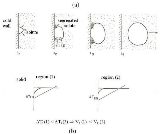
Fig. 4. (a) Schematic illustration of the mechanism of detachment of nuclei from the surface of the cooling slope; (b) temperature profiles in the liquid in the solidification front, for an alloy with partition coefficient  $K < 1$
