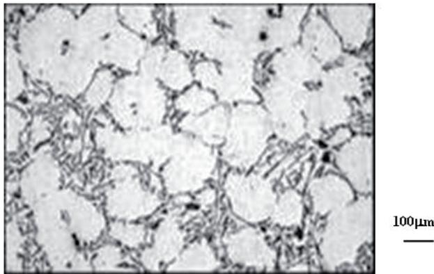
Fig. 11. Thixocast microstructure of A356 alloy produced by electromagnetic stirring + re-heating at 580°C/15min
