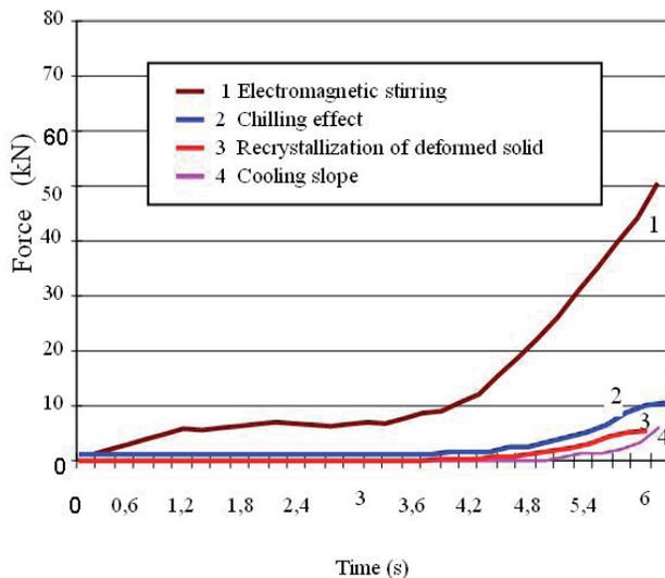
Fig. 14. Force x time during thixoforging of A356 alloy in the semi-solid state produced from raw material obtained by different techniques
