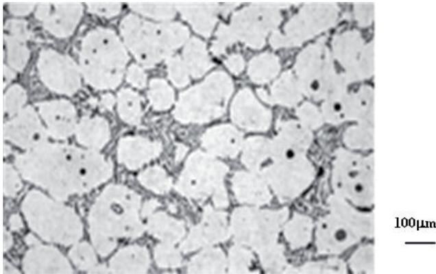
Fig. 8. Thixocast microstructure of A356 alloy produced by stimulating chilling effect + re-heating at 580°C/15min
