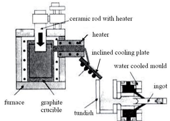
Fig. 1. Schematic illustration of horizontal continuous casting apparatus with inclined cooling plate used in the experiments
