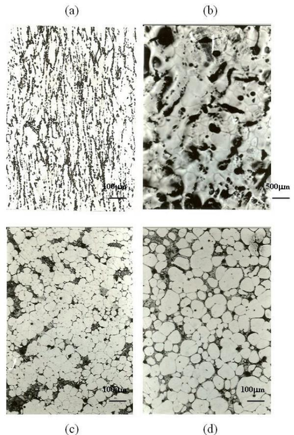
Fig. 12. Microstructures of A356 alloy in different conditions: (a) cold deformed (80% true def.); (b) heated at 580°C/2 min; (c) heated at 580°C/5 min; (d) heated at 580°C/15 min
