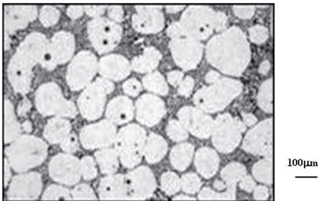
Fig. 5. Thixocast microstructure of A356 alloy produced by continuous casting with cooling plate + re-heating at 580°C/15min
