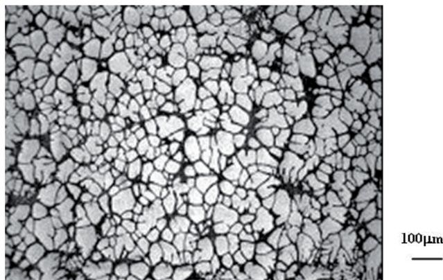
Fig. 3. Microstructure of A356 alloy obtained by continuous casting with cooling plate
