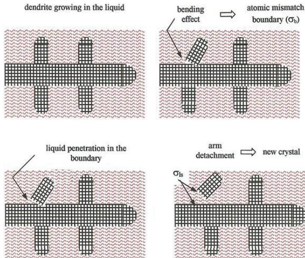
Fig. 10. Schematic illustration of detachment of secondary dendrite arms by liquid penetration in high energy boundary formed by bending due to stirring in the liquid
