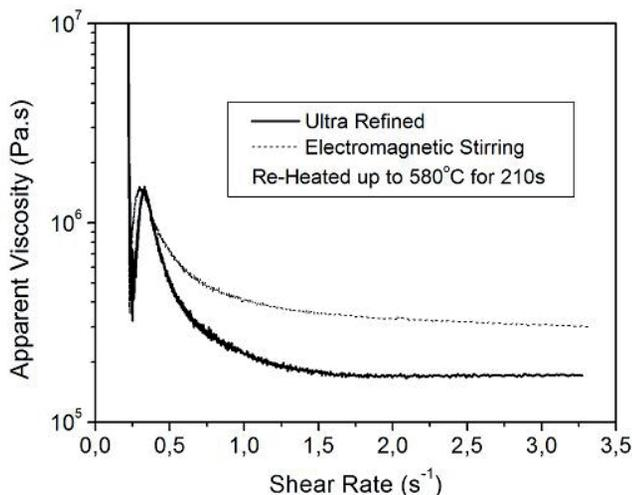
Fig. 13. Apparent viscosity x shear rate of A356 alloy in the semi-solid state produced from ultra-refined material (intensive initial nucleation) and from electromagnetic stirred material (fragmented dendrites)
