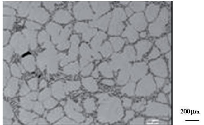
Fig. 9. Microstructure of A356 alloy obtained by electromagnetic stirring of the liquid while solidifying
