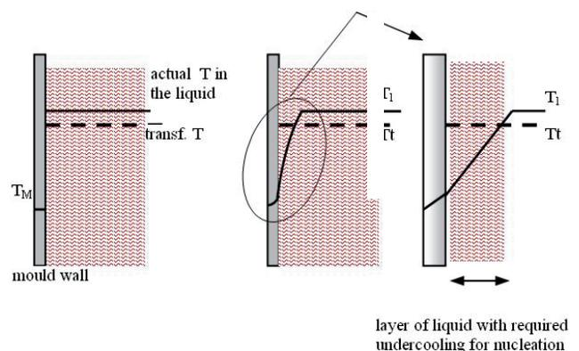
Fig. 7. Schematic illustration of the thermal conditions close to mould walls when a liquid with low superheating is poured in a mould with high thermal conductivity
