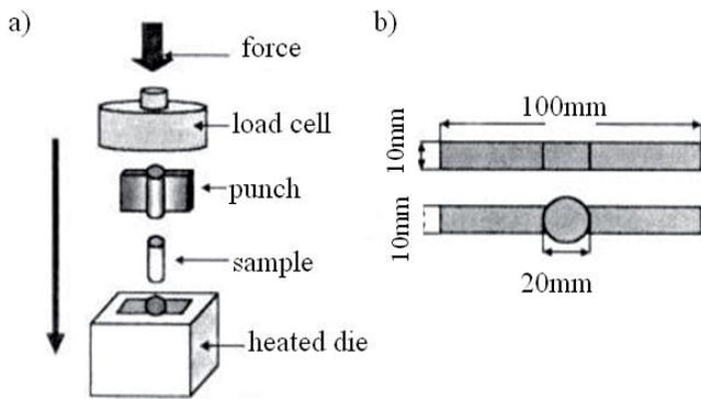
Fig. 2. Schematic illustration of (a) the thixoforging operation; (b) dimensions of final product
