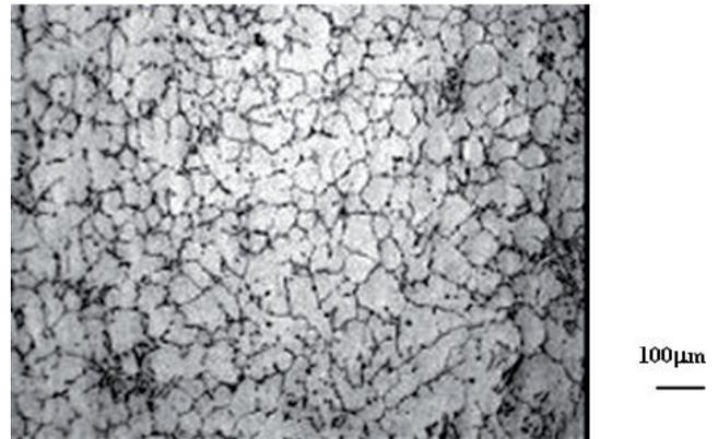
Fig. 6. Microstructure of A356 alloy obtained by pouring with low superheating in a cold metallic mould
