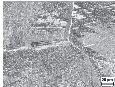
Fig. 6. Microstructure after melting and casting from a ceramic underlay (Degussa) [1,2]
