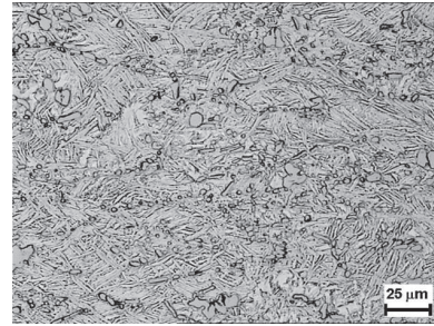
Fig. 5. Microstructure after casting from a graphite melting crucible, with a subsequent rolling [3]
