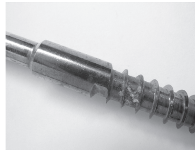
Fig. 3. Screw coated by Nanocrystalline Diamond coatings after 18 months in human body
