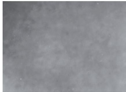
Fig. 1. Structure of Co<sub>70,5</sub>Fe<sub>2,5</sub>Mn<sub>4</sub>Mo<sub>1</sub>Si<sub>9</sub>B<sub>15</sub> amorphous alloy at quenched state, with characteristic contrast (TEM, thin foil, magnification 80 000x)
