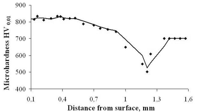
Fig. 7. Change of the X38CrMoV5-3 steel surface layer microhardness after remelting using the 2.0 kW laser
