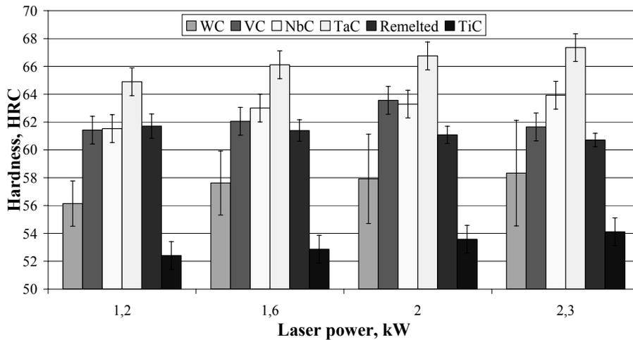
Fig. 10. Changes of the average hardness of the X38CrMoV5-3 steel surface layer after alloying with carbides using the variable power laser
