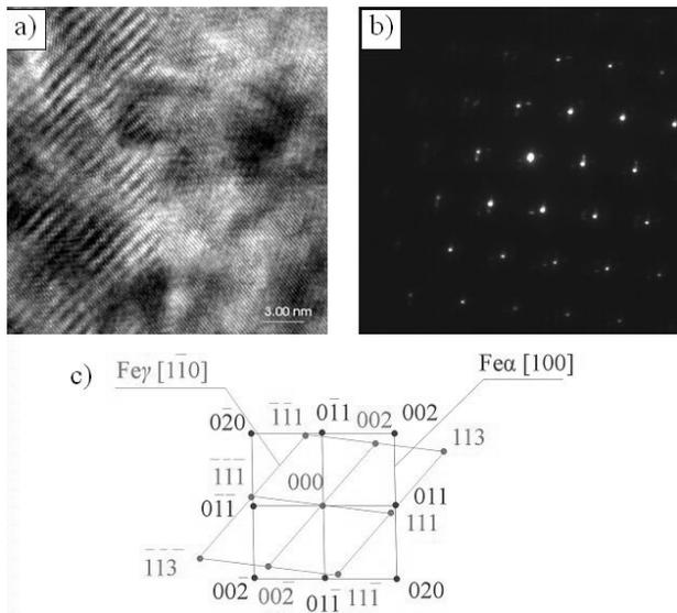
Fig. 21. a)TEM image of the X38CrMoV5-3 after remelting, b) diffraction pattern of area shown in a, c) part of solution for diffraction pattern shown in b
