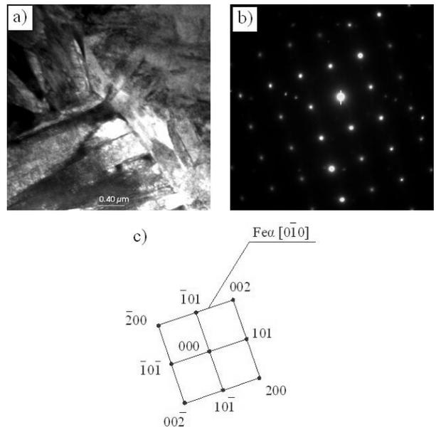
Fig. 20. a)TEM image of the X38CrMoV5-3 after standard heat treatment, b) diffraction pattern of area shown in a, c) part of solution for diffraction pattern shown in b
