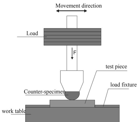
Fig. 4. Schematic diagram of the device for abrasion wear resistance tests of the surface layers in the metal-metal arrangement
