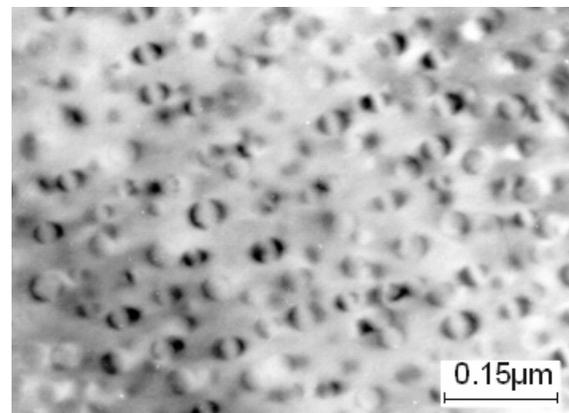
Fig. 1. Structure of the alloy after solution heat treatment and aging at 715°C/150h. Coherent spheroidal  $\gamma'$  phase precipitates in the matrix
