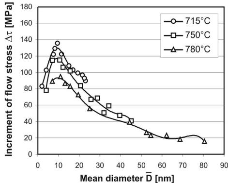
Fig. 7. Relations between increased flow stress and mean diameter of  $\gamma'$  precipitates
