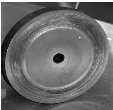
Fig. 5. View on samples and counter-samples after measurement of the rate of attrition a) samples b) counter-sample
