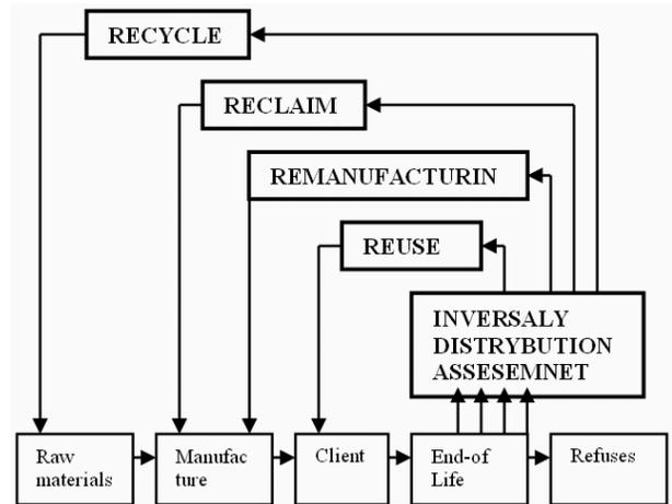
Fig. 1 Diagram of recovery
