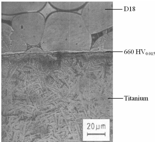
Fig. 3. Microstructure of titanium – D18 pseudoalloy of tungsten joint
