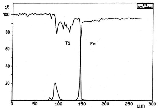
Fig. 4. Titanium – Armco iron joint a) microstructure and microhardness, b) linear distribution of iron and titanium
