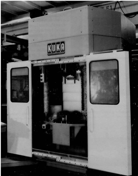
Fig. 1. Friction welding machine
