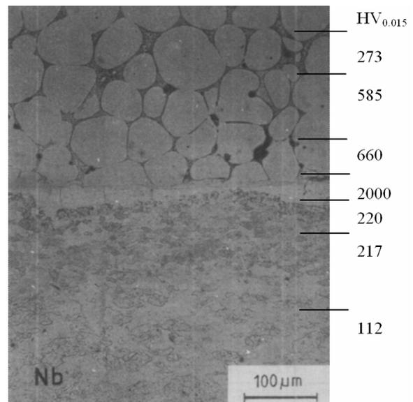
Fig. 2. Microstructure and microhardness of Ni - D18 pseudoalloy of tungsten joint
