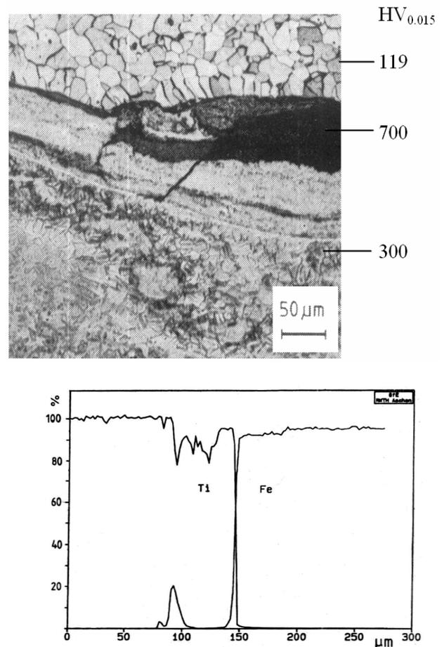
Fig. 4. Titanium – Armco iron joint a) microstructure and microhardness, b) linear distribution of iron and titanium
