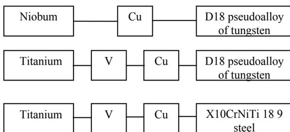
Fig. 5. Interlayer systems in niobium and titanium joints
