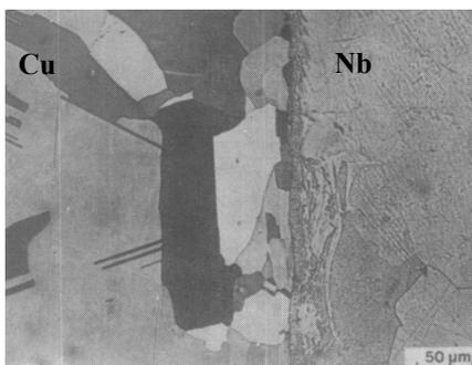
Fig. 6. Microstructure of niobium – D18 pseudoalloy of tungsten joint with copper interlayer
