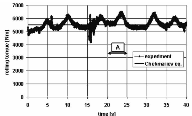
Fig. 2. Distributions of the rolling torque in the oval-circle pass
