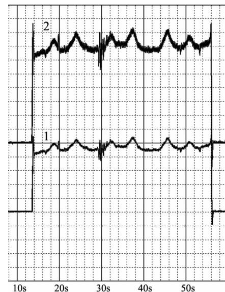
Fig. 1. Change of electromechanical signal for the main drive motor: 1 - values of current intensity measured for the computation of rolling torque, 2 - values of current intensity measured for the computation of rolling power
