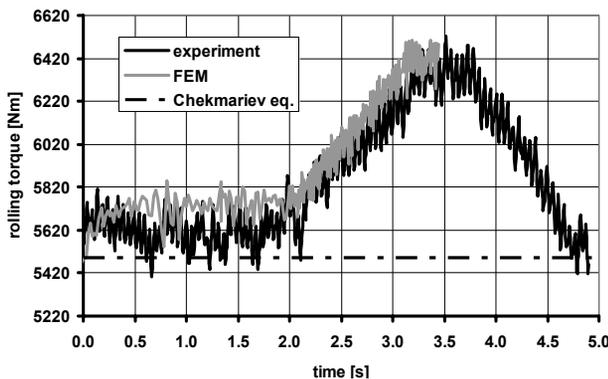
Fig. 4. Comparison of theoretical and experimental rolling torque values
