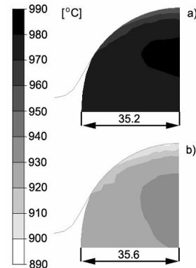
Fig. 6. Distribution of temperature and variations in band width in the plane of exist from the deformation zone: a) initial temperature of 970°C; b) initial temperature of 920°C
