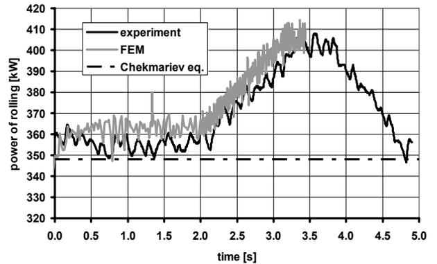
Fig. 5. Comparison of theoretical and experimental rolling power values
