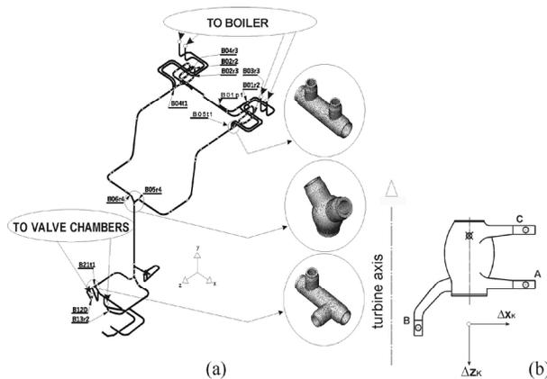
Fig. 4. Example of the re-superheated steam pipeline - (a); valve chamber draft with dislocation directions indicated - (b)
