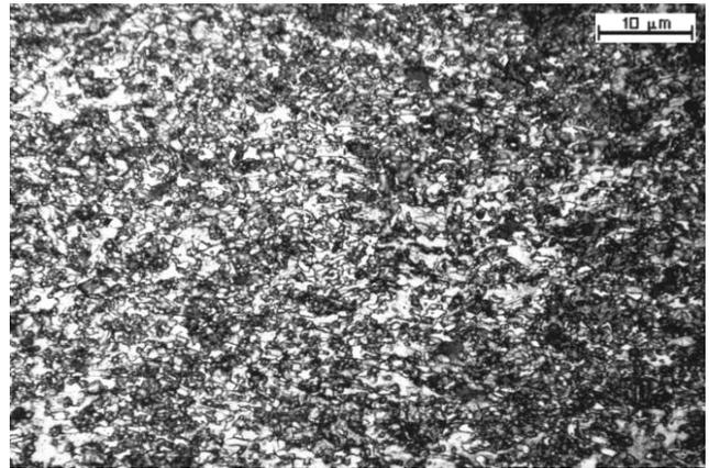
Fig. 4. Ferritic – bainitic structure with the retained austenite of the thermo-mechanically processed steel isothermally held for 600 s at a temperature of 400°C
