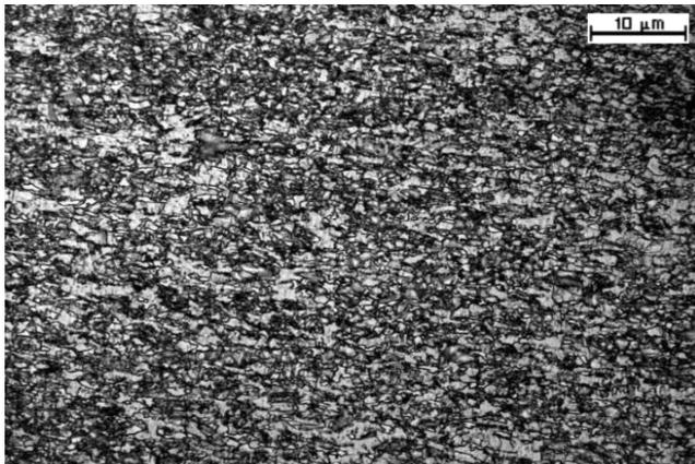
Fig. 3. Ferritic – bainitic structure with the retained austenite of the thermo-mechanically processed steel isothermally held for 600 s at a temperature of 300°C
