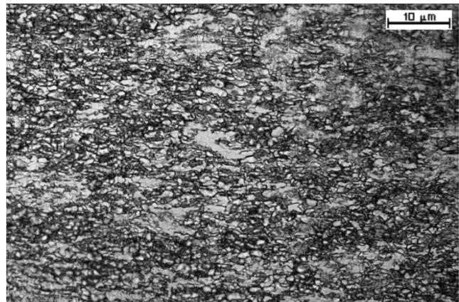
Fig. 5. Ferritic – bainitic structure with the retained austenite of the thermo-mechanically processed steel isothermally held for 600 s at a temperature of 500°C
