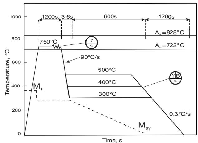
Fig. 1. Schematic representation of the thermomechanical processing of the investigated steel,  $M_s$  – martensite start temperature of the steel,  $M_{s\gamma}$  – martensite start temperature of the austenite with increased carbon concentration
