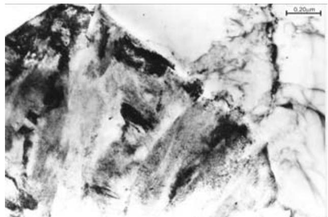
Fig. 6. Structure of bainitic ferrite with the retained austenite located between its laths and on a boundary of bainite and ferrite with an increased dislocation density
