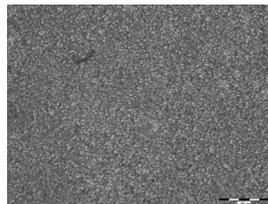
Fig. 5. AZ91 + T4 after rolling and ECAP
