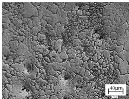
Fig. 4. AZ91+T4 after rolling (3<sup>rd</sup> pass)
