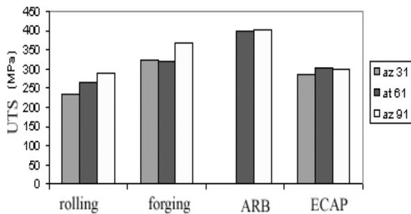
Fig. 13. UTS of Mg alloys at different technologies [8]
