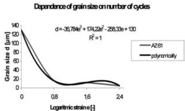
Fig. 11. Grain size on logarithmic strain dependence of AZ91 alloy at ARB process
