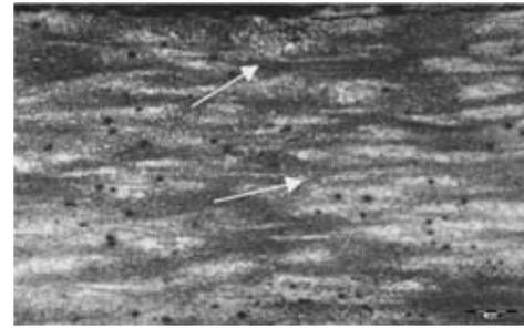
Fig. 9. Final microstructure AZ91 after 5<sup>th</sup> pass at ARB process
