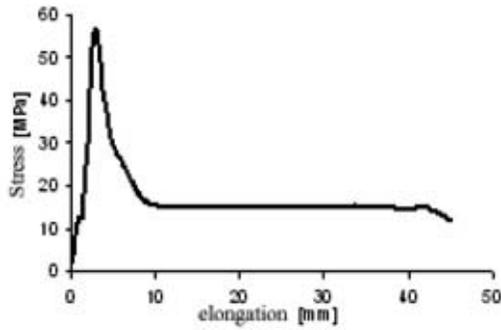
Fig. 7. Diagram of ECAPed AZ91 alloy after hot tensile test
