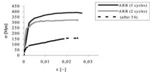
Fig. 10. Mechanical properties of AZ91 at the temperature 360°C
