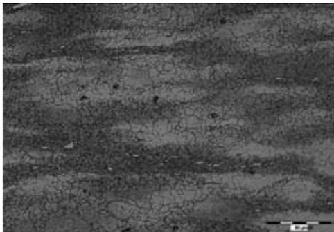
Fig. 8. Final microstructure of AZ61 after 3<sup>rd</sup> pass at ARB process
