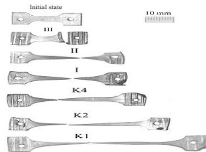
Fig. 6. Samples of AZ91+T4 alloy after ECAP and hot tensile test
