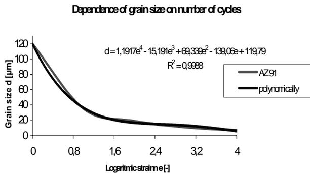
Fig. 12. Grain size on logarithmic strain dependence of AZ61 alloy at the ARB process
