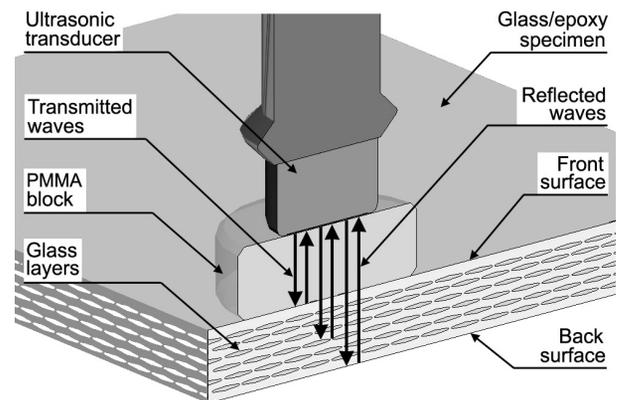
Fig. 1. Scheme of the ultrasonic testing (pulse-echo technique)
