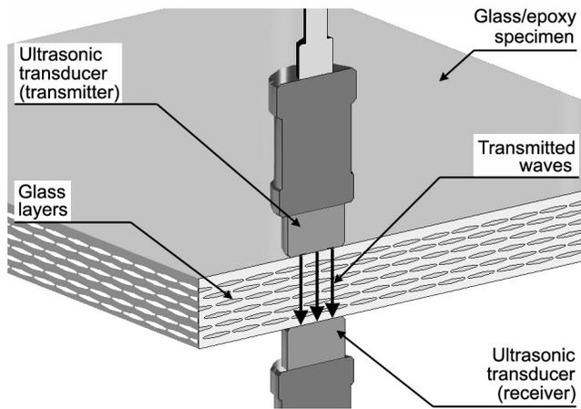
Fig. 2. Scheme of the ultrasonic testing (through-transmission technique)
