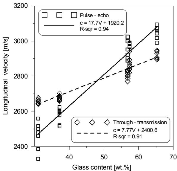
Fig. 3. Ultrasonic wave velocity vs. fiber content
