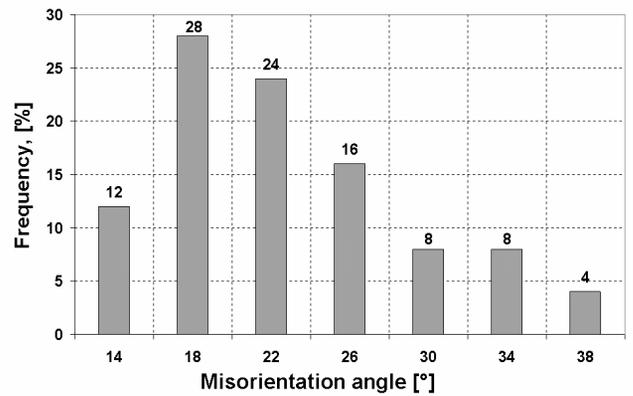
Fig. 4. Statistical distribution of the coarse-grained austenite's misorientation angle after elongation of  $A_{3\text{mm}}=60\%$
