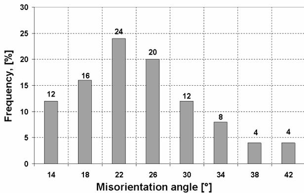
Fig. 6. Statistical distribution of the austenite grain's misorientation angle after elongation of  $A_{3mm}=200\%$
