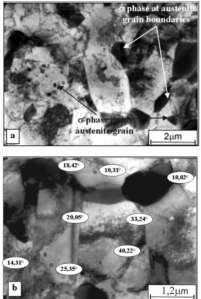
Fig. 5. The structure of steel subjected to tension up to the elongation of  $A_{3\text{mm}}=200\%$ , a - Region of austenite and  $\sigma$  phase precipitation, b - Misorientation angles between austenite grains in the vicinity of  $\sigma$  phase precipitates
