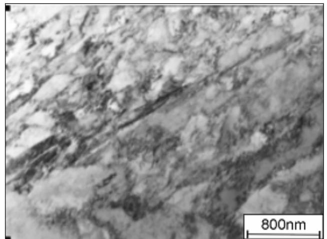
Fig. 2. The structure of steel subjected to tensioned at  $T=850^\circ\text{C}$  with the velocity of  $v_t=15\times 10^{-3}\text{mm/s}$ , to the elongation of  $A_{3\text{mm}}=60\%$ . Primary austenite region
