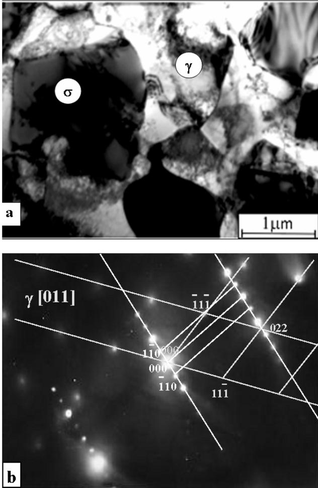
Fig. 3. The structure of steel subjected to tension at  $T=850^\circ\text{C}$  with the velocity of  $v_f=15 \times 10^{-3} \text{ mm/s}$ , to the elongation of  $A_{3\text{mm}}=60\%$ , a - austenite region formed as a result of transition from ferrite and  $\sigma$  phase precipitates, b - diffraction from the centre of figure 3 a
