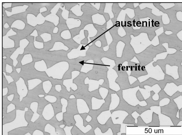
Fig.1. Structure of the X2CrNiMoN22-5-3 ferritic-austenitic steel after solution heat treatment from a temperature of  $T=1250^\circ\text{C}$  with soaking time of 60 minutes and cooling in water. Austenite surface fraction is  $A_A=30\pm 0.5\%$
