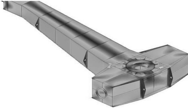
Fig. 6. Distribution of Huber - Mises stress steering carriage
