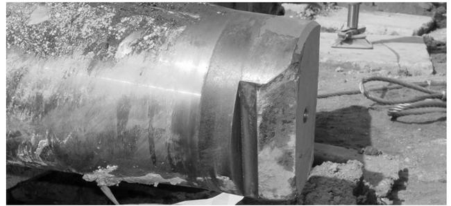
Fig. 4. Damaged halfshaft of steerable carriage
