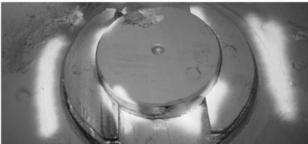
Fig. 7. Halfshaft end - protection against slip out
