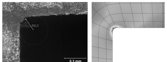
Fig. 10. Groove edge curvature radius  $r = 0.2$  mm on specimen's left side, plastic strain zone on groove's bottom
