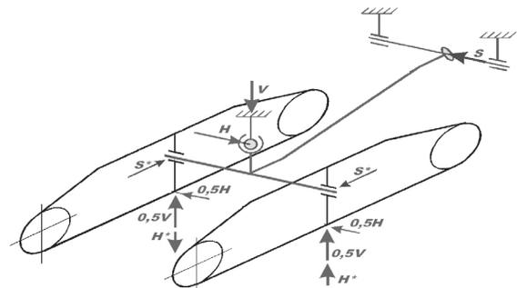
Fig. 5. Forces acting on caterpillar unit during turn
