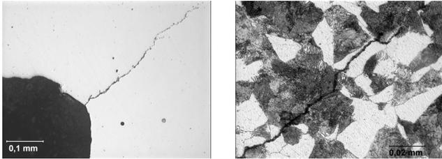
Fig. 11. Fatigue crack propagating along ferrite and pearlite grains
