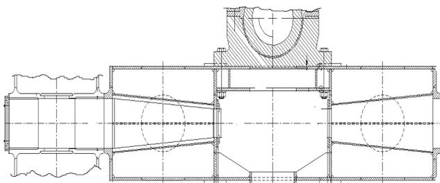
Fig. 3. Halfshaft mounting in carriage structure.
