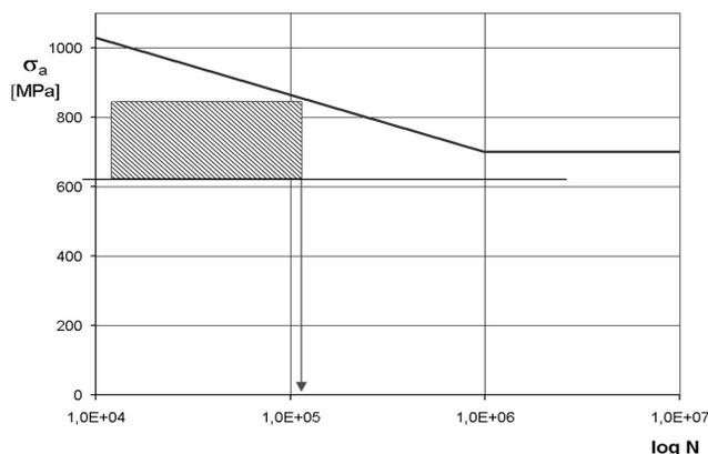
Fig. 12. Wöhler diagram for steel 40HM with marked limited fatigue strength region for radius  $r = 0.2$  mm in halfshaft grooves
