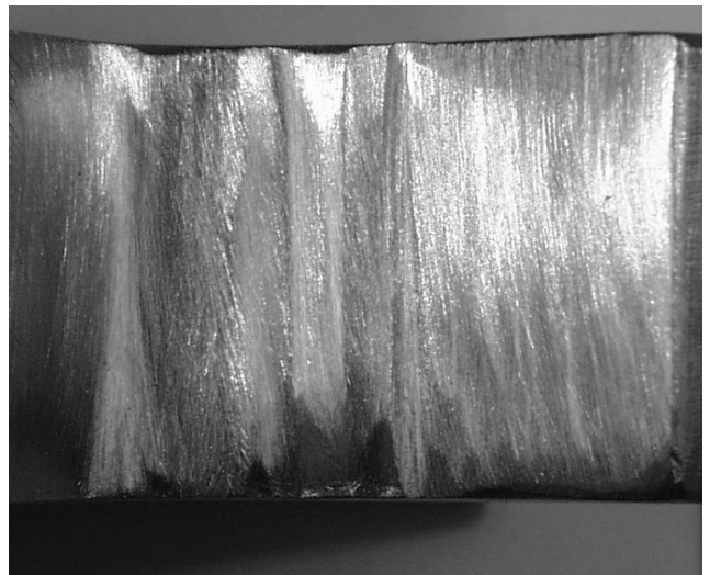
Fig. 17. Macrostructure of the weld after corrosion test; heat input 3.0 kJ/mm; no pitting corrosion
