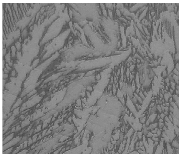
Fig. 7. Microstructure of the weld; heat input HI = 4.5; ferrite - dark phase, austenite - bright phase; ferrite (α) volume fraction 47%
