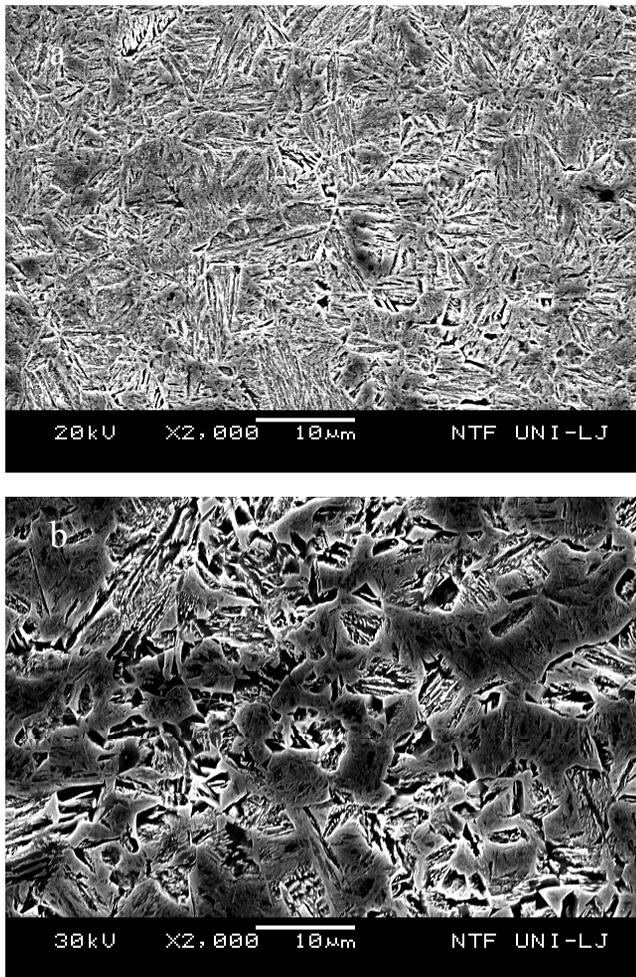
Fig. 6. SEM micrographs of Jominy specimens of Mn-Mo steel at near the quenched end (a), and 40 mm from the quenched end of the sample (b)
