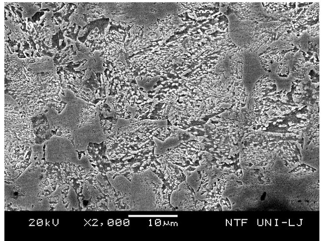
Fig. 5. SEM micrographs of Jominy specimens of Cr-Mo steel at near the quenched end (a), and 40 mm from the quenched end of the sample (b)
