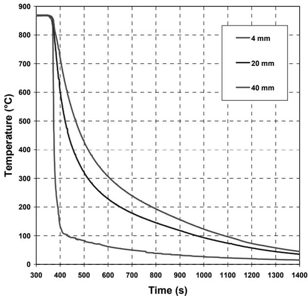
Fig. 3. Change of temperature during cooling of the Jominy specimen for Mn-Mo steel at different distances from the specimen end-face
