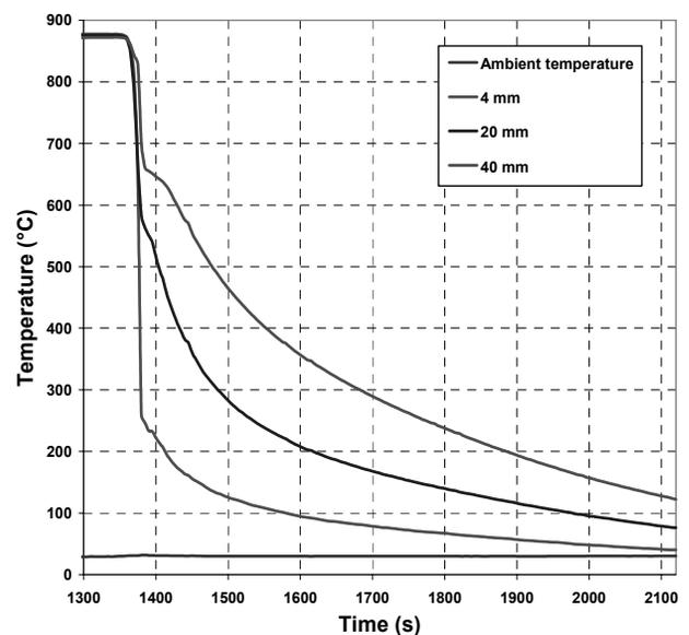
Fig. 2. Change of temperature during cooling of the Jominy specimen for Cr-Mo steel at different distances from the specimen end-face
