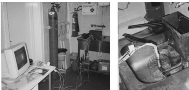
Fig. 1. Equipment and quenching system for the hardenability testing by Jominy method
