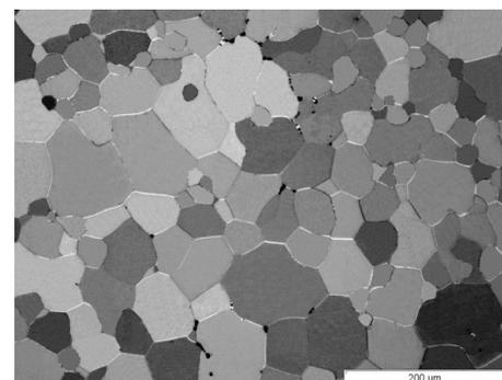
Fig. 3. Solid solution grains in WE54 alloy after solutioning
