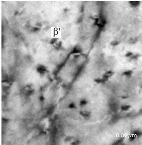
Fig. 4. The  $\beta'$  precipitates after ageing at 250°C for 4h
