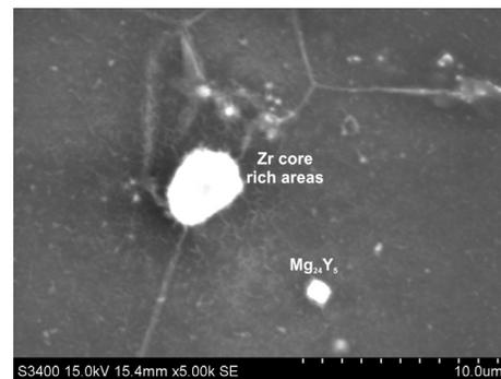
Fig. 2. Zirconium rich core areas and precipitate of  $Mg_{24}Y_5$  phase in WE54 alloy in as cast condition, SEM
