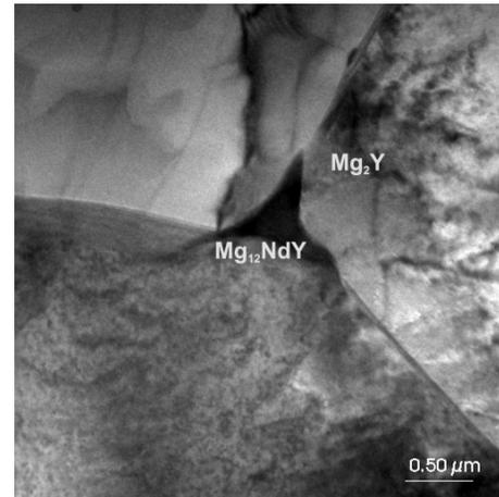
Fig. 1. Precipitates of  $Mg_2Y$  and  $Mg_{12}YNd$  phases in  $\alpha$ -Mg matrix of WE54 alloy in as cast condition, TEM
