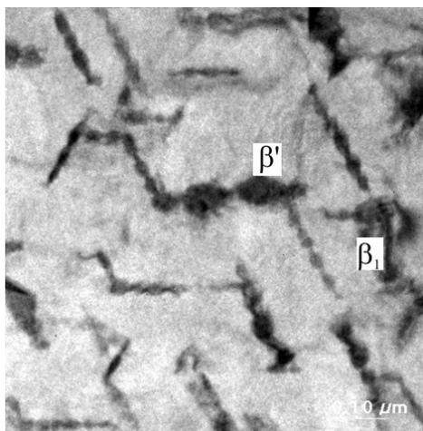
Fig. 6. Network of  $\beta'$  and  $\beta_1$  precipitates after ageing at 250°C for 96h
