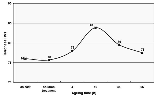
Fig. 8. Change of hardness during ageing at 250°C
