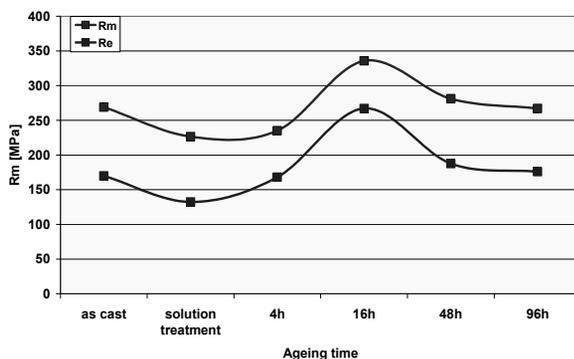
Fig. 10. Change of a tensile strength and yield point during ageing at 250°C (temperature 200°C)
