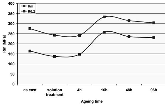
Fig. 9. Change of a tensile strength and yield point during ageing at 250°C (ambient temperature)
