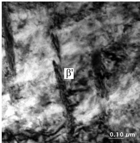
Fig. 5. The  $\beta'$  precipitates after ageing at 250°C for 16h
