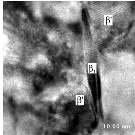
Fig. 7. The  $\beta_1$  precipitate between two  $\beta'$  precipitates in WE54 alloy after ageing at 250°C for 96h
