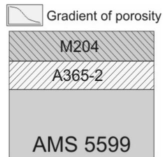
Fig. 2. The conception of TBC system with a gradient of porosity
