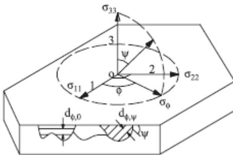
Fig. 4. Model of the in-plane elastic residual stresses (method  $\sin^2\Psi$ )
