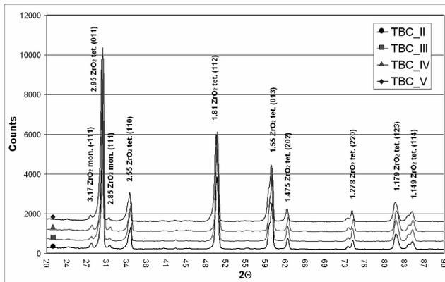
Fig. 5. The results of XRD phases identification from the top surface of gradient TBC.
