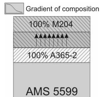
Fig. 3. The conception of TBC system with a gradient of chemical composition
