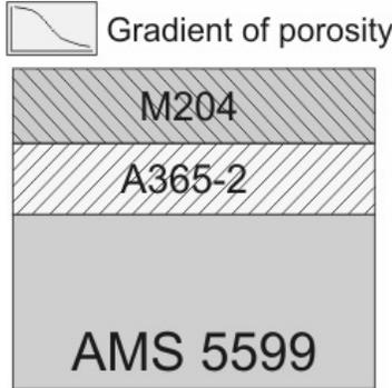
Fig. 4. The conception of TBC system with a gradient of porosity
