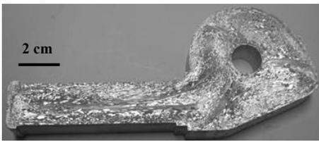
Fig. 6. The specimen with both seam welds and transverse weld;  $T_B=510^{\circ}\text{C}$ ,  $V_R=15\text{ mm/s}$ ,  $T_E=520^{\circ}\text{C}$
