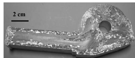
Fig. 2. The specimen with both seam welds and transverse weld;  $T_B=470^\circ\text{C}$ ,  $V_R=10\text{mm/s}$ ,  $T_E=500^\circ\text{C}$
