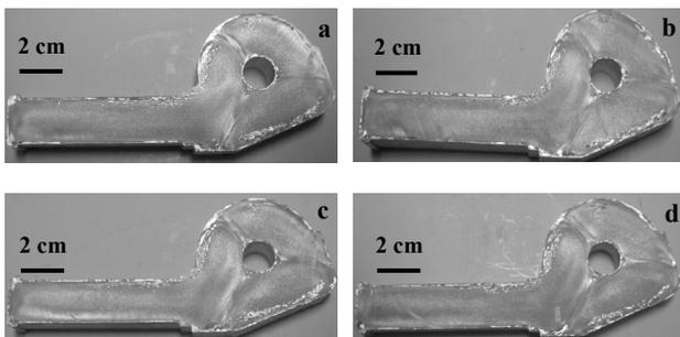
Fig. 1. The specimens with only seam welds (without transverse weld): a)  $T_B=430^\circ\text{C}$ ,  $V_R=10\text{mm/s}$ ,  $T_E=475^\circ\text{C}$ ; b)  $T_B=430^\circ\text{C}$ ,  $V_R=10\text{mm/s}$ ,  $T_E=440^\circ\text{C}$ ; c)  $T_B=450^\circ\text{C}$ ,  $V_R=15\text{mm/s}$ ,  $T_E=475^\circ\text{C}$ ; d)  $T_B=430^\circ\text{C}$ ,  $V_R=15\text{mm/s}$ ,  $T_E=475^\circ\text{C}$
