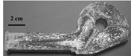
Fig. 9. The specimen with both seam welds and transverse weld;  $T_B=490^{\circ}\text{C}$ ,  $V_R=10\text{ mm/s}$ ,  $T_E=520^{\circ}\text{C}$
