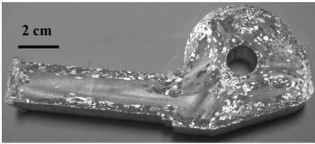
Fig. 3. The specimen with both seam welds and transverse weld;  $T_B=490^{\circ}\text{C}$ ,  $V_R=10\text{ mm/s}$ ,  $T_E=500^{\circ}\text{C}$
