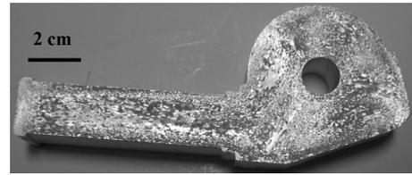
Fig. 8. The specimen with both seam welds and transverse weld;  $T_B=510^{\circ}\text{C}$ ,  $V_R=10\text{ mm/s}$ ,  $T_E=560^{\circ}\text{C}$ .
