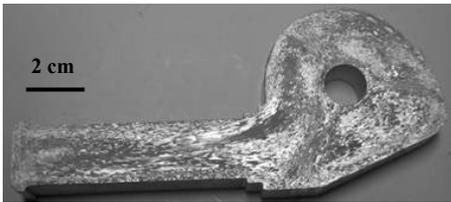
Fig. 5. The specimen with both seam welds and transverse weld,  $T_B=490^{\circ}\text{C}$ ,  $V_R=6\text{ mm/s}$ ,  $T_E=520^{\circ}\text{C}$
