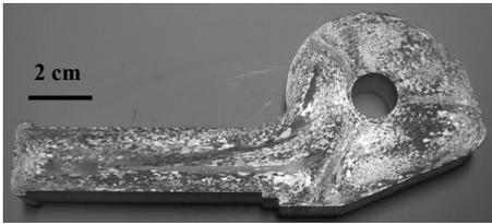
Fig. 4. The specimen with both seam welds and transverse weld;  $T_B=490^{\circ}\text{C}$ ,  $V_R=15\text{ mm/s}$ ,  $T_E=520^{\circ}\text{C}$
