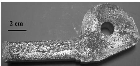
Fig. 7. The specimen with both seam welds and transverse weld;  $T_B=510^{\circ}\text{C}$ ,  $V_R=4\text{ mm/s}$ ,  $T_E=560^{\circ}\text{C}$
