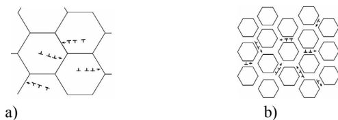
Fig. 1. Grain size (a) act as obstacles for lattice dislocation in primary poly-crystals, (b) as softening of building elements, which carry plastic flow in nano-crystalline materials [1, 2]
