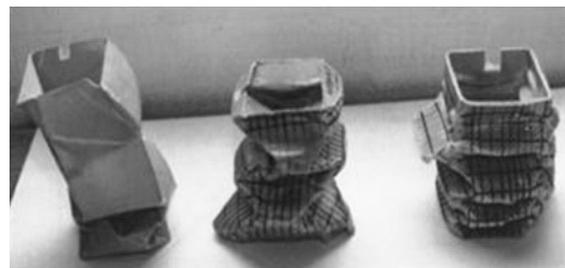
Fig. 9. Thickness effect on the collapse modes for (a) GRP tubes and (b) Kevlar tubes
