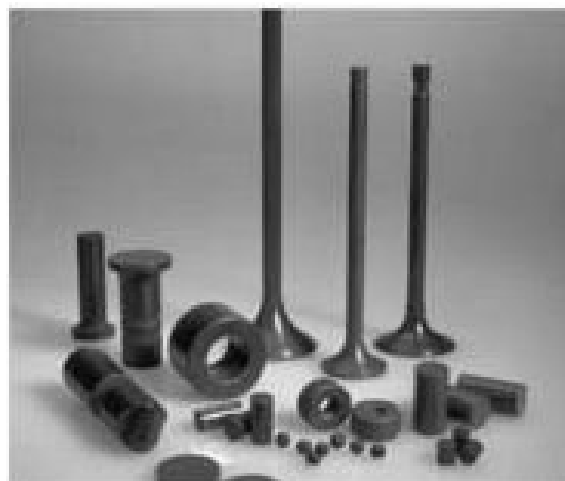
Fig. 10. Silicon nitride wear parts for engines
