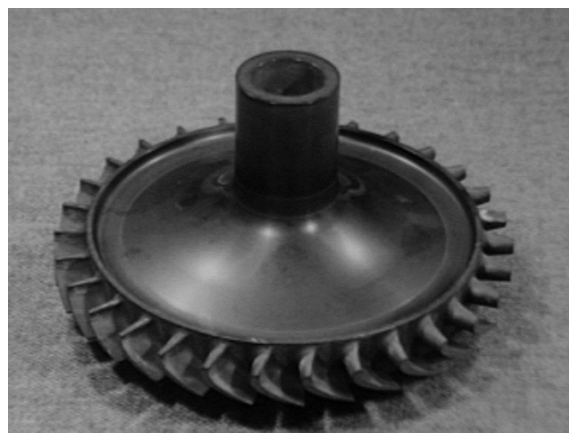
Fig. 9. Silicon nitride turbocharger rotor
