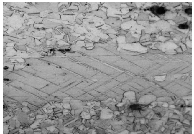
Fig. 7. Structure of industrial bronze type CuSn6Zr after hot rolling, shearing bands with slip lines and inclusions, (x1000)
