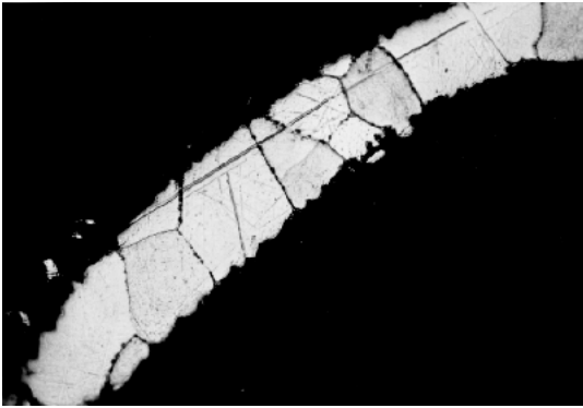
Fig. 5b. Exemplary image of an extremely brittle gauze (3000 hours) longitudinal microsection, optical microscope -300x [8,9]
