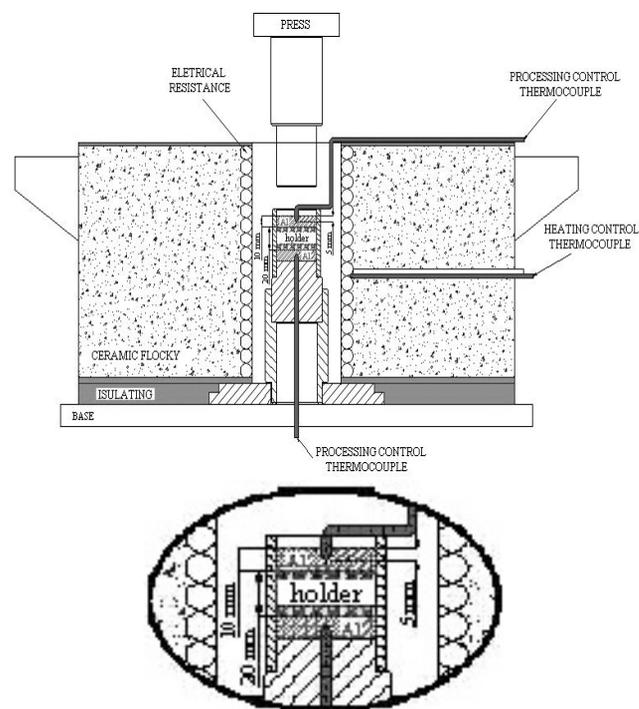
Fig. 1. Schematic representation of the infiltration process of semi-solid thixotropic A2011 into a layer of space holder particles, to produce porous metallic material
