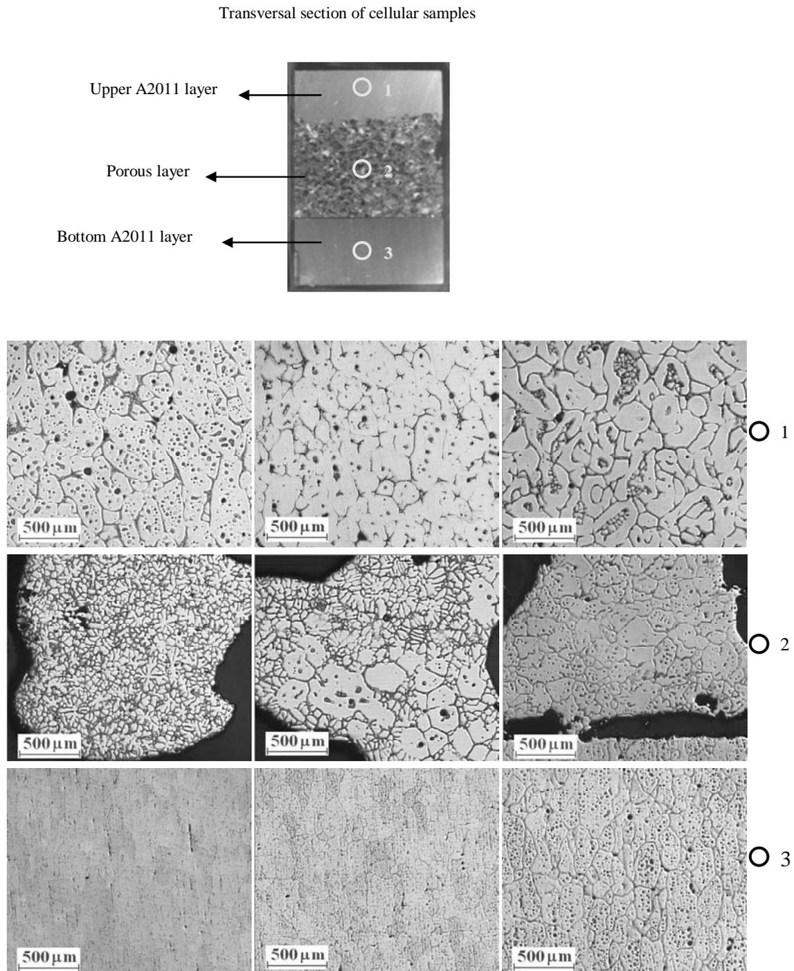
Fig. 8. Microstructures of cellular A2011 produced by thixoforming into a layer of space holder particles with coarse dimensions. Thixoforming temperatures: (a)  $T = 620^{\circ}\text{C}$ ; (b)  $630^{\circ}\text{C}$ ; (c)  $640^{\circ}\text{C}$ . Regions shown according to indication
