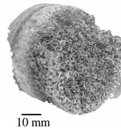
Fig. 3. General aspect of cellular A2011 alloy produced by thixoforming at  $T = 620^{\circ}\text{C}$  into a layer of fine space holder particles
