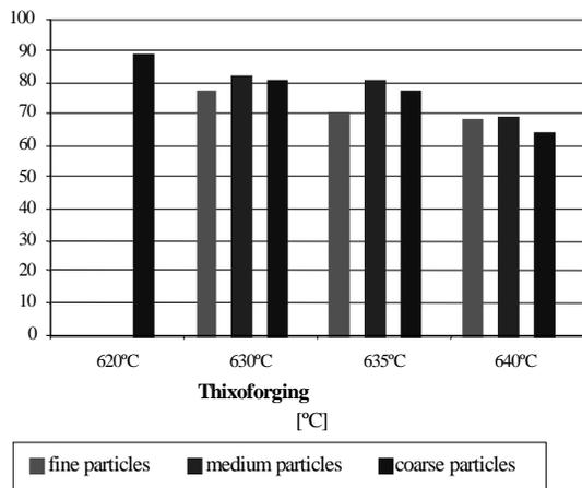
Fig. 9. Voids content in cellular A2011 produced by thixoforming at different temperatures into a layer of space holder particles of different dimensions
