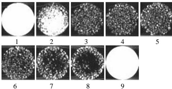
Fig. 7. Tomography images of cellular A2011 produced by thixoforming at 620°C, into a layer of fine particles of space holders. Sections from top (1) to bottom surfaces (9) of cylindrical samples
