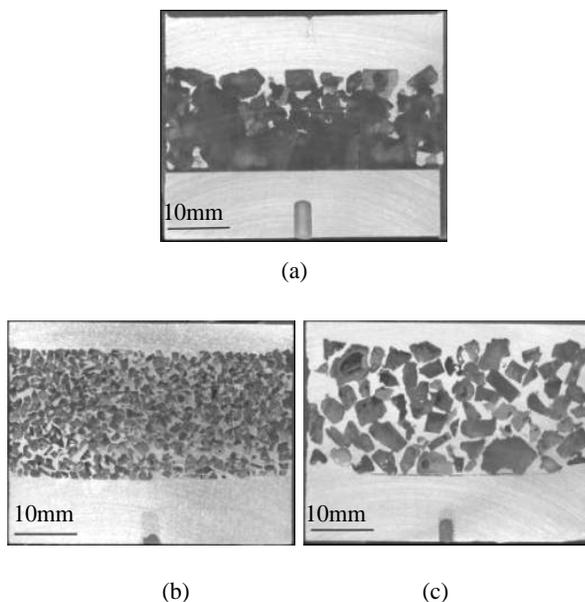
Fig. 5. Transversal sections of typical samples of cellular A2011 alloy produced by thixoforming in different conditions: (a)  $T = 620^{\circ}\text{C}$ , coarse space holder particles; (b)  $T = 640^{\circ}\text{C}$ , fine space holder particles; (c)  $T = 640^{\circ}\text{C}$ , coarse space holder particles
