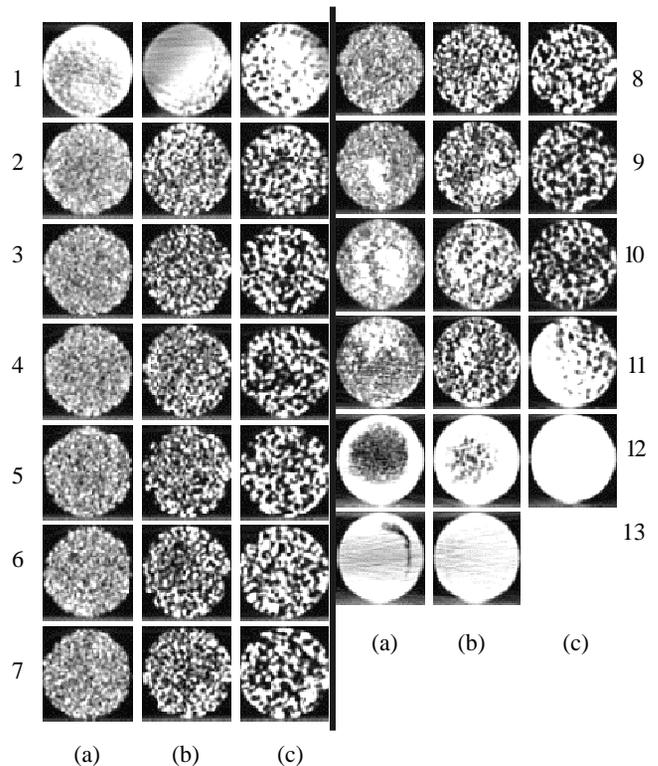
Fig. 6. Tomography images of cellular A2011 produced by thixoforming at  $640^{\circ}\text{C}$ , into a layer of space holder particles with dimensions: (a) fine; (b) medium; (c) coarse
