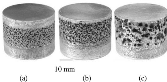
Fig. 2. General aspect of typical cellular A2011 alloy produced by thixoforming into a layer of space holder particles. a) and b) fine particles; c) coarse particles. Thixoforming conditions: (a)  $T = 620^{\circ}\text{C}$ ; (b) and (c)  $T = 640^{\circ}\text{C}$
