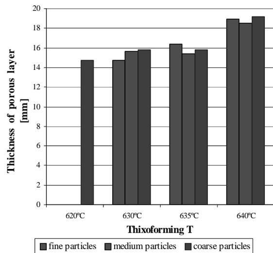
Fig. 4. Thickness of porous material x processing parameters - evaluation of infiltration ability of thixotropic A2011 into a layer of space holder particles with different dimensions
