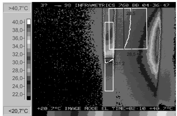
Fig. 9. Thermograph of sample subjected to 1 190 000 fatigue cycles 1 second after heating
