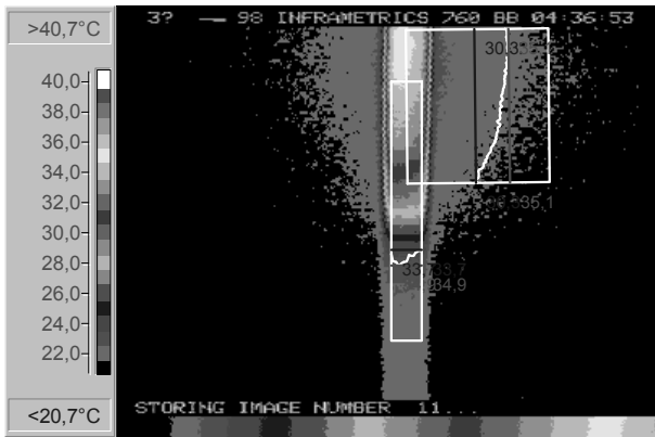
Fig. 11. Thermograph of sample subjected to 1 190 000 fatigue cycles 20 seconds after heating
