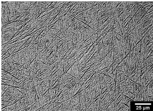
Fig. 18. Microstructure of a cast from the Ti64 alloy, after the heat processing [1,2,6,10]
