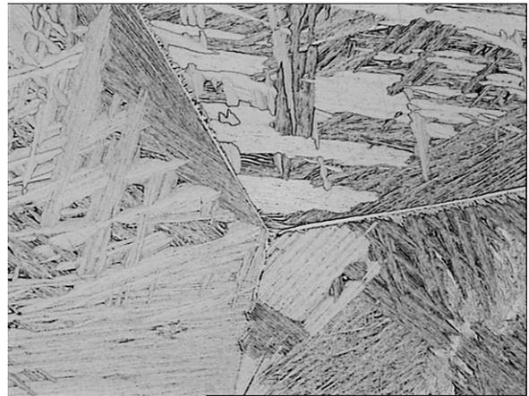
Fig. 15. Microstructure of a cast, after melting the Ti64 alloy in a v plasma furnace [1,2,6,9]
