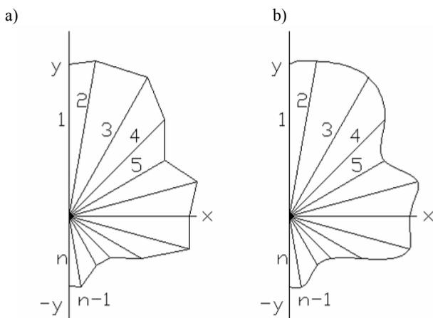
Fig. 1. Schematic representation of creation a figure in the plane, (x – y): a) line-segments, b) spline segments
