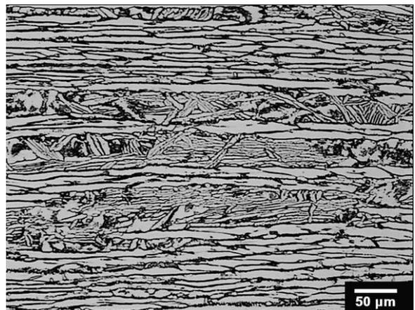
Fig. 16. Microstructure of rolling shaped component of certified alloy Ti64 [1,2,6,7,8]
