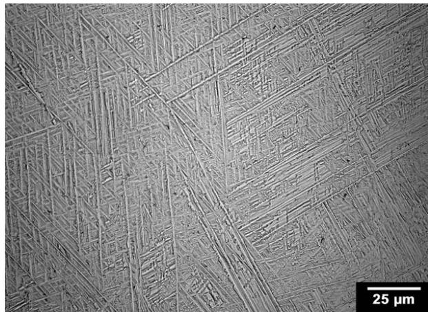
Fig. 17. Microstructure of a cast of the Ti64 alloy, into a copper crystalliser [1,2,6,9]
