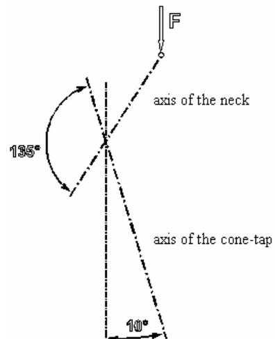
Fig. 13. Loading scheme of the implant model
