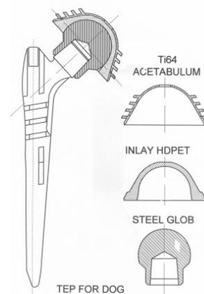
Fig. 3. Design of a TEP for im-, planting into experimental animals [1]
