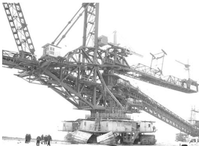
Fig. 3. Breakdown of dumping conveyor's steerable carriage
