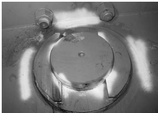
Fig. 10. Halfshaft end - protection against slip out
