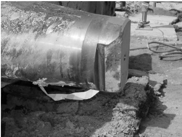
Fig. 7. Damaged halfshaft of steerable carriage
