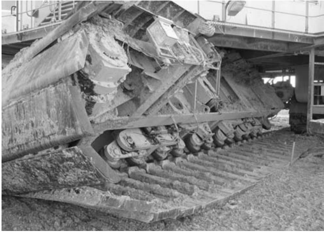
Fig. 6. Breakdown of one carriage: results of steerable carriage breakdown
