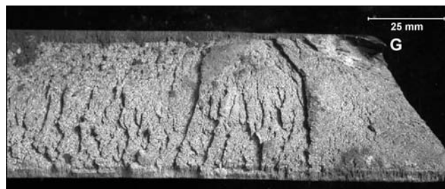
Fig. 16. Element 2. Magnified fragment from fig. 15 (visible plastic deformation in point G)
