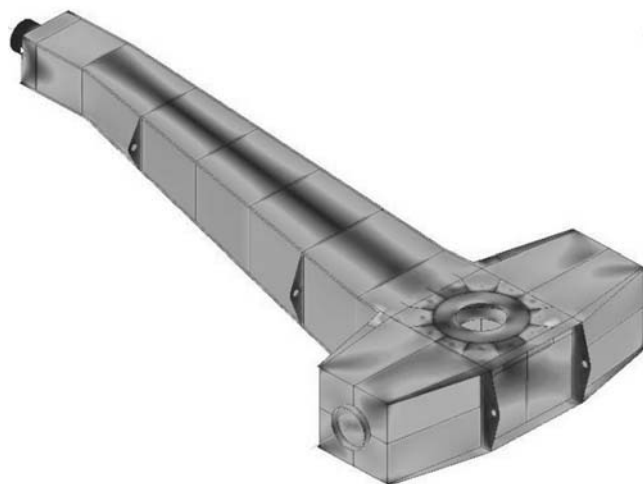
Fig. 9. Distribution of Huber - Misses stress in dumping conveyor's steering carriage
