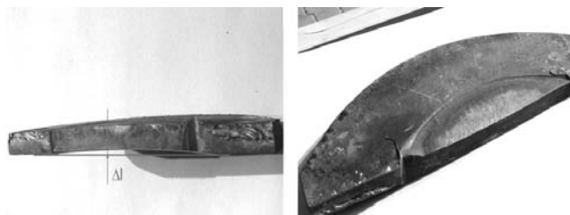
Fig. 11. Deformed elements (plates) protecting against halfshaft slip out
