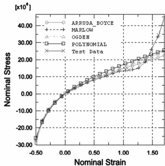
Fig. 2 Selection the forms of strain energy potentials
