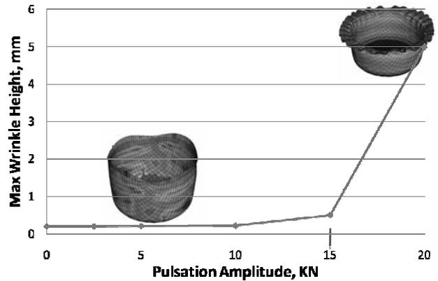
Fig. 16. Effect of BHF pulsation amplitude on wrinkling height
