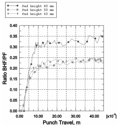
Fig. 10. Variation of the BHF/PF ratio with pad height
