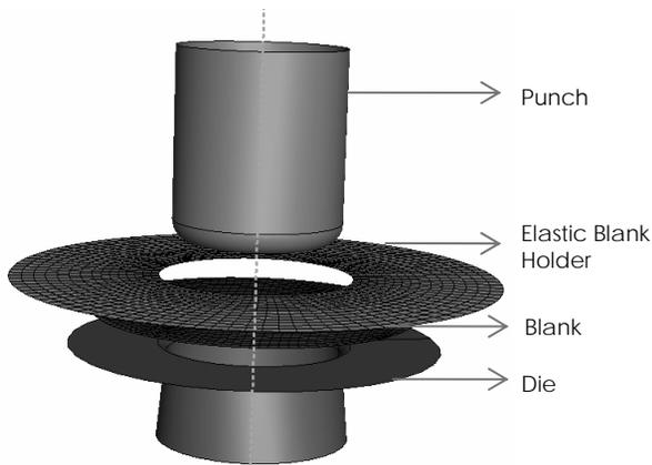
Fig. 3. An elastic (pliable) blank-holder model
