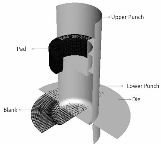
Fig. 1. Model of the friction actuated BH technique
