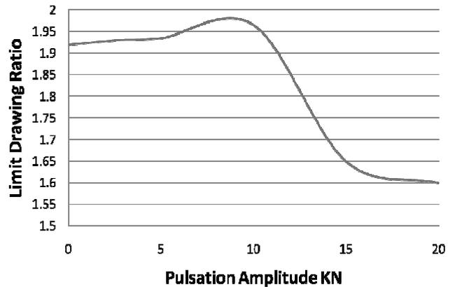
Fig. 17. Variation of the LDR with the BHF amplitude
