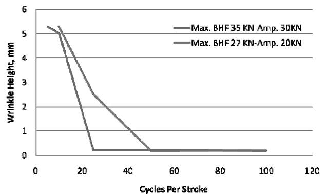
Fig. 12. Effect of the BHF frequency on wrinkling
