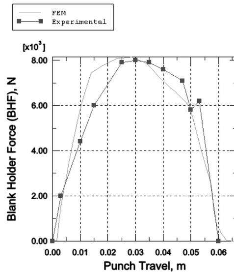
Fig. 5. Finite element predicted BHF compared to the experimental one [4]
