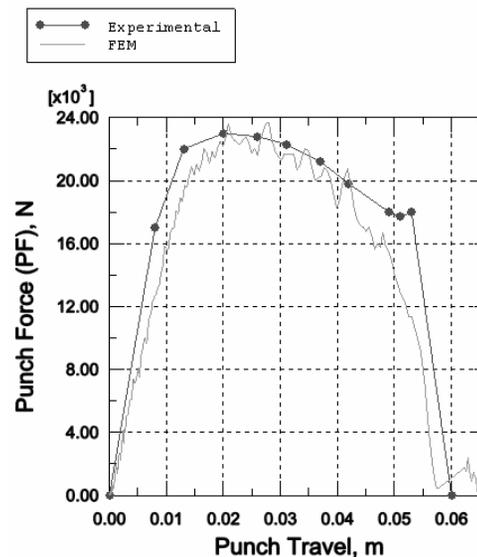
Fig. 6. Finite element predicted PF compared to the experimental one [4]
