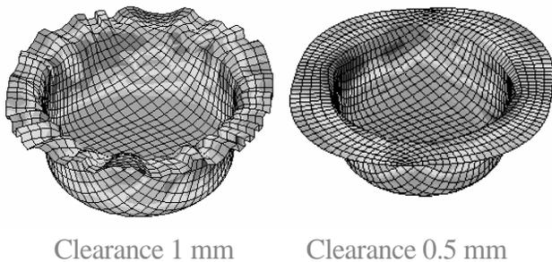
Fig. 8. Effect of excessive clearance on wrinkling
