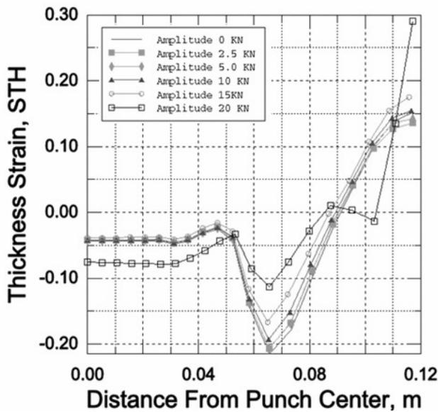
Fig. 15. Effect of BHF pulsation amplitude on thickness strain
