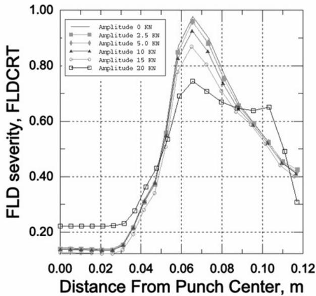
Fig. 14. Effect of BHF pulsation amplitude on deformation severity
