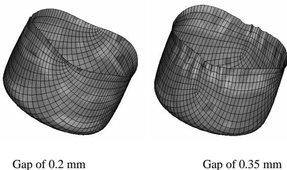
Fig. 11. Effect of gap height on the wrinkling of elastic BH
