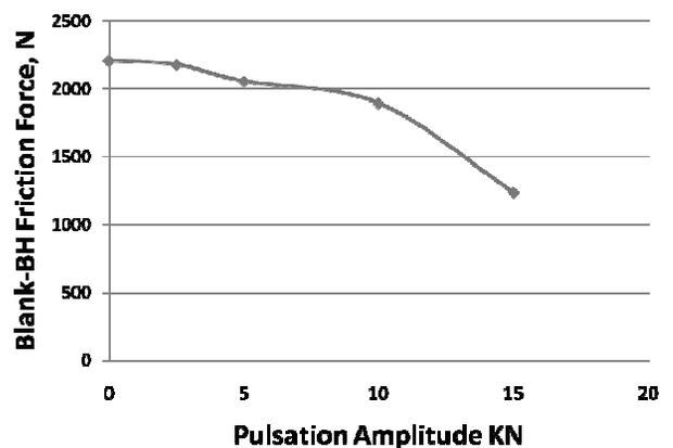
Fig. 13. Effect of the BHF pulsation amplitude on friction force
