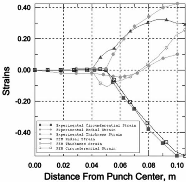
Fig. 7. Predicted strain distributions as compared to experimental ones [4]
