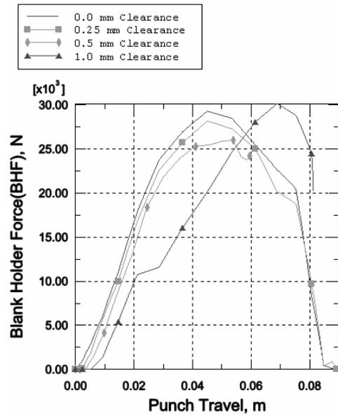
Fig. 9. Effect of clearance on BHF
