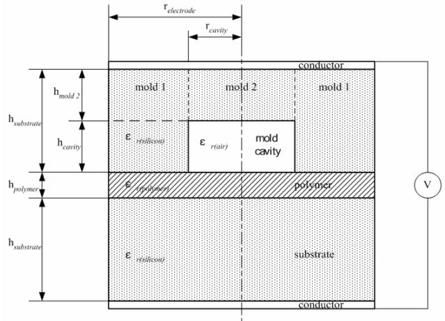
Fig. 6. Simplified equivalent model for the proposed capacitance detection unit
