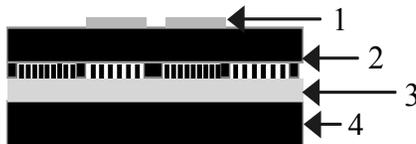
Fig. 5. Schematic of capacitive sensing device, where (1) is the platinum top sensing electrodes; (2) the silicon imprint mold; (3) the polymer layer; and (4) the silicon substrate
