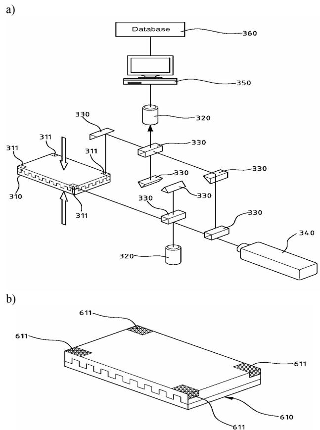
Fig. 2. Optical method for monitoring the mold deformation [22] a-system setup, b-mold with markings
