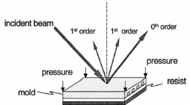
Fig. 3. Schematic of NIL characterization using TRDS [29]
