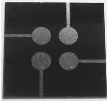
Fig. 4. Photograph of sensing electrodes on the imprint mold unit
