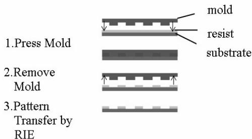
Fig. 1. Schematic diagram of the nanoimprint lithography process
