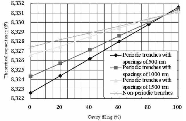
Fig. 7. Correlation between theoretical capacitance and cavity filling for various patterns
