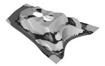
Fig. 9. Defect free double attached part with cut-off lines
