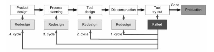
Fig. 1. Flow chart of process planning and die design in traditional CAD environment
