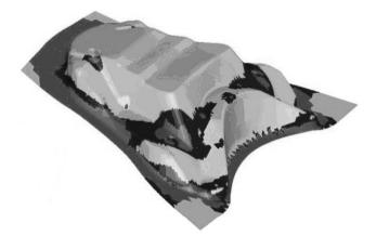
Fig. 8. Cracks arising at die radius due to excessive stretching
