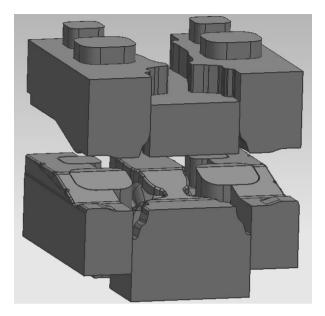
Fig. 12. The solid model of the complete tool assembly
