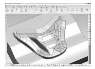
Fig. 10. Solid model of the punch created from the reference geometry using the AF-UG interface
