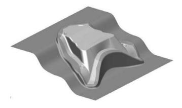
Fig. 6. Modified reference surface to derive the tool surfaces
