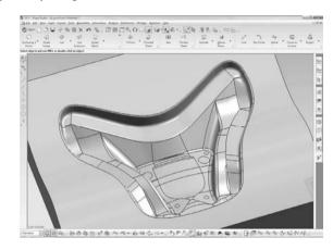
Fig. 11. Solid model of the die created from the reference geometry using the AF-UG interface
