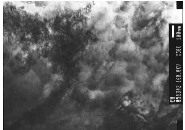
Fig. 5b. Microstructure of the deformed nanocrystalline copper; TEM
