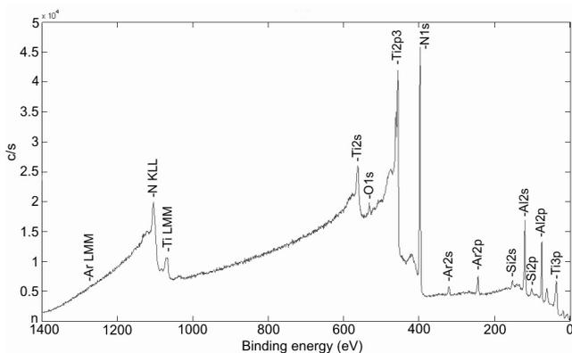
Fig. 8. Surface spectrum of (Ti,Al,Si)N gradient coating deposited on the  $\text{Al}_2\text{O}_3$  oxide tool ceramic reinforced with SiC whiskers obtained with XPS method (area of analysis: 2 mm x 0.8 mm rectangle)
