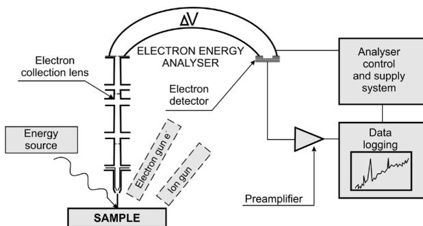
Fig. 1. Schematic diagram of X-Ray Photoelectron Spectroscopy (XPS)
