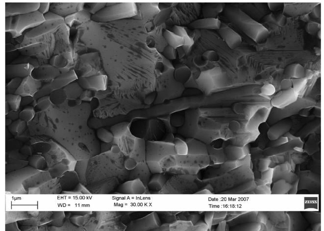
Fig. 2. Structure of the  $\text{Al}_2\text{O}_3$  oxide tool ceramic reinforced with SiC whiskers
