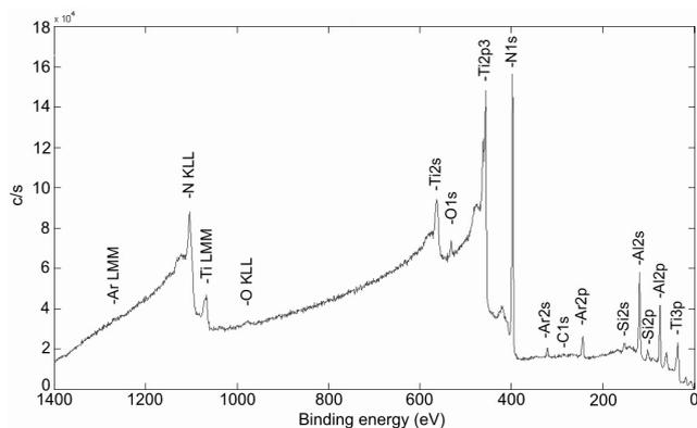
Fig. 7. Surface spectrum of (Ti,Al,Si)N gradient coating deposited on the  $\text{Al}_2\text{O}_3$  oxide tool ceramic reinforced with SiC whiskers obtained with XPS method (area of analysis: 0.4 mm circle)
