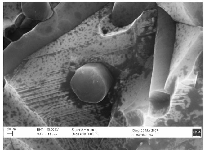
Fig. 3. Structure of the  $\text{Al}_2\text{O}_3$  oxide tool ceramic reinforced with SiC whiskers
