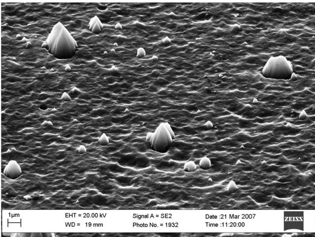
Fig. 5. Topography of the gradient  $(\text{Ti,Al,Si})\text{N}$  coating surface, deposited on the  $\text{Al}_2\text{O}_3+\text{SiC}_{(w)}$  oxide tool ceramic
