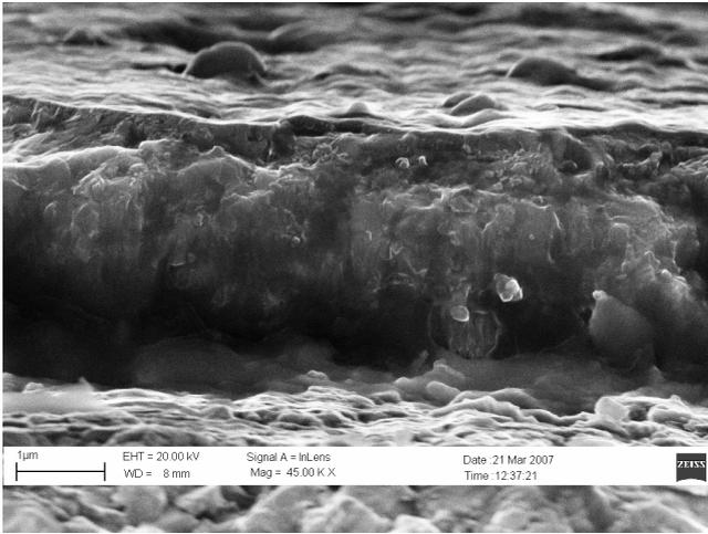
Fig. 4. Fracture surface of the gradient  $(\text{Ti,Al,Si})\text{N}$  coating deposited onto the  $\text{Al}_2\text{O}_3+\text{SiC}_{(w)}$  oxide tool ceramic
