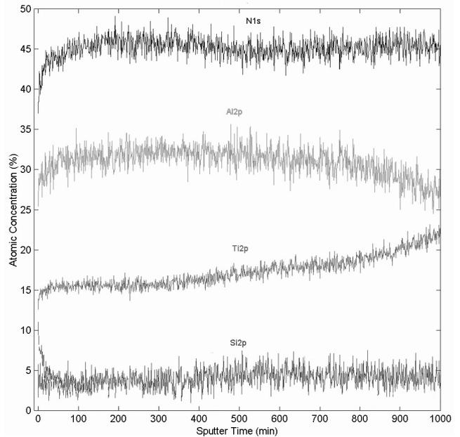
Fig. 6. Depth profile of the chemical composition obtained with XPS method on the  $(\text{Ti,Al,Si})\text{N}$  coating
