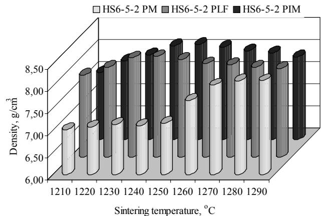
Fig. 3. Density versus sintering temperature of high speed-steel formed by powder injection moulding (PIM), pressureless forming (PLF) and compacted and sintered (PM)
