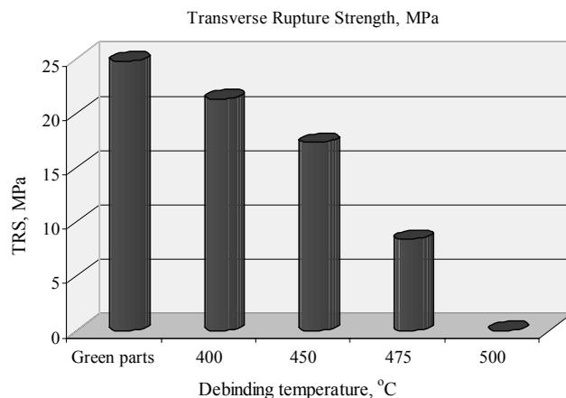
Fig. 1. Mechanical properties of green and brown parts deduced from the three point bending test
