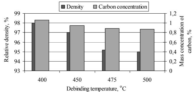
Fig. 2. Relative density and carbon concentration of samples sintered at 1240°C after thermal debinding at temperature: a) 400, b) 450, c) 475, d) 500°C
