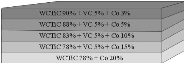
Fig. 5 Scheme of TGM sample type A
