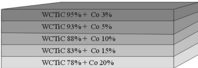
Fig. 6 Scheme of TGM sample type B
