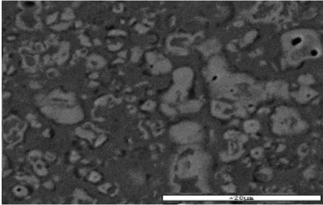
Fig. 10 Microstructure of WCTiC+VC+Co gradient material, central layer
