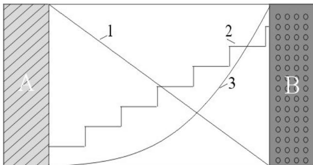
Fig. 1 Type of gradient: 1- linear; 2- stepped; 3- parabolical
